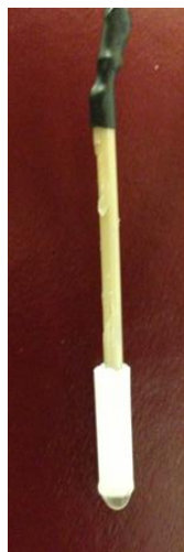
Figure 3-3. Schematic of the 5-mm Gold Electrode Ruggedized with a Porous Frit (left); Gold Electrode with Frit (right)
