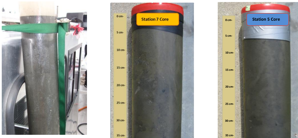
Figure 3-6. Core Sample in Polycarbonate Liners (left); Cores Sectioned into 5 cm Segments (right)
