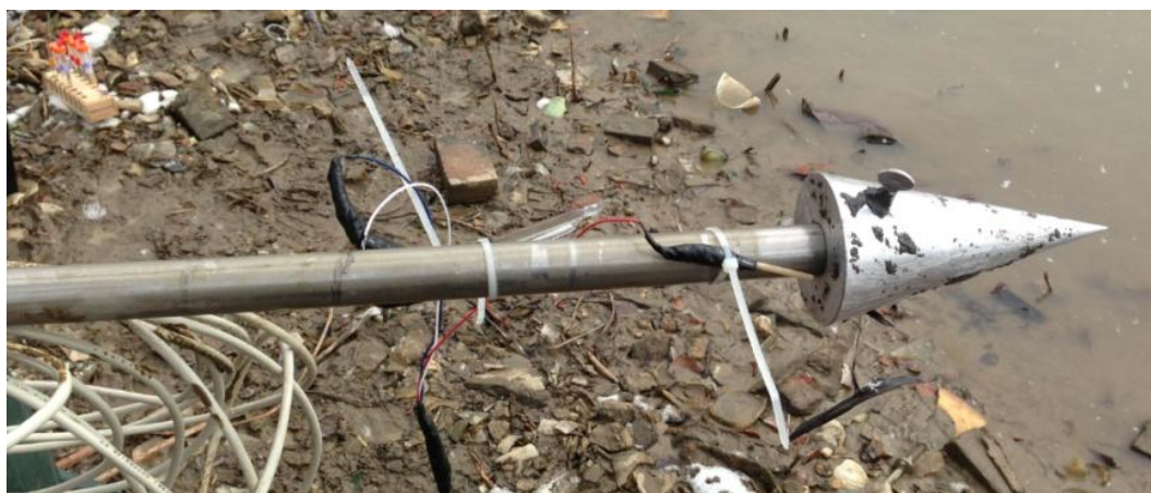
Figure 3-4. A Steel Rod with an Aluminum Tip was Fabricated to Shelter the Electrode Tip
