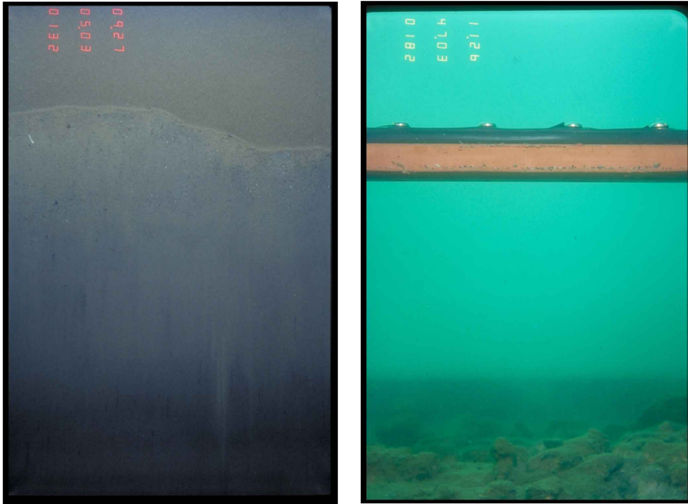
Figure 5-15. Sediment profile images from SE Loch showing the two different sediment types found: a). The sediments at Station B were typical of the majority of locations; b) Station K had minimal penetration due to the hard cobble bottom (Scale: Width of images = 15 cm).
