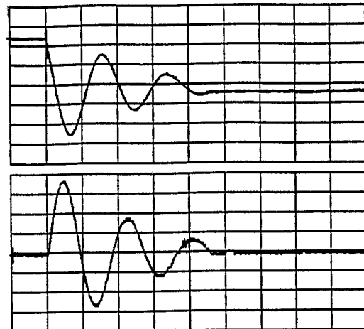
Figure 10. Two type F capacitors in series. Upper trace: Voltage 200 V/div. Lower trace: Current 800 A/div. Horizontal axis: 50 \mu s/div.
