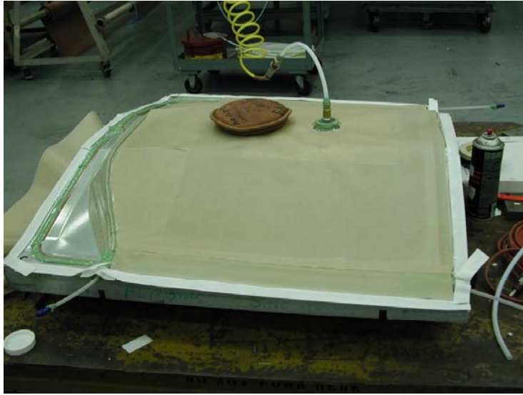
Figure 75. Second Bag Lay-up Showing Porous Armalon
