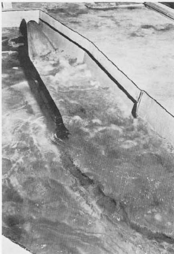
Photograph 15. Flow through original design stilling basin with 2 rows of baffle piers Discharge, 7,500 cfs Tailwater elev, 923.9 (normal)
