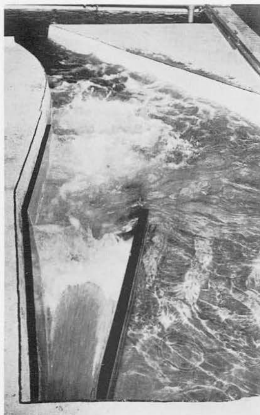
Photograph 25. Flow through original design stilling basin with 7.5-ft end sill, right wall shortened 108 ft Discharge, 10,800 cfs Tailwater elev, 926.8 (normal)
