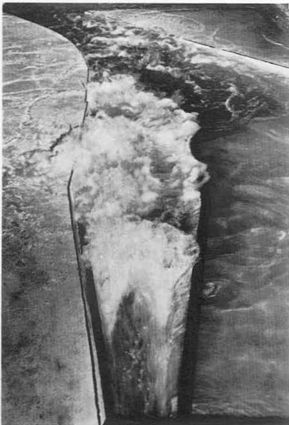
Photograph 4. Downstream view of flow through original design stilling basin Discharge, 11,750 cfs Tailwater elev, 939.0 (normal +5.0 ft)
