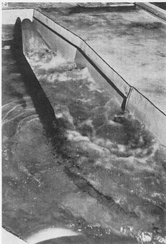
Photograph 11. Flow through original design stilling basin Discharge, 7,500 cfs Tailwater elev, 923.9 (normal)
