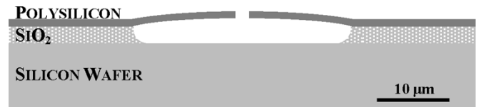
Fig. 1. Bisection of the polysilicon shell-type micromechanical resonator.
