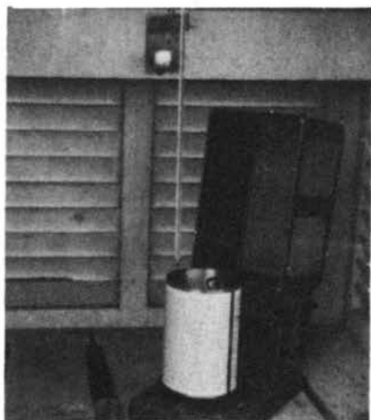
FIGURE 2 THERMOGRAPH AND THERMOMETER
