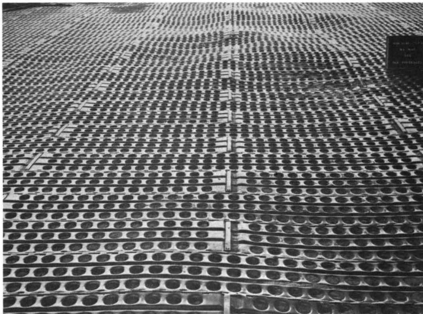
M6 mat in section 4 after 966 coverages
