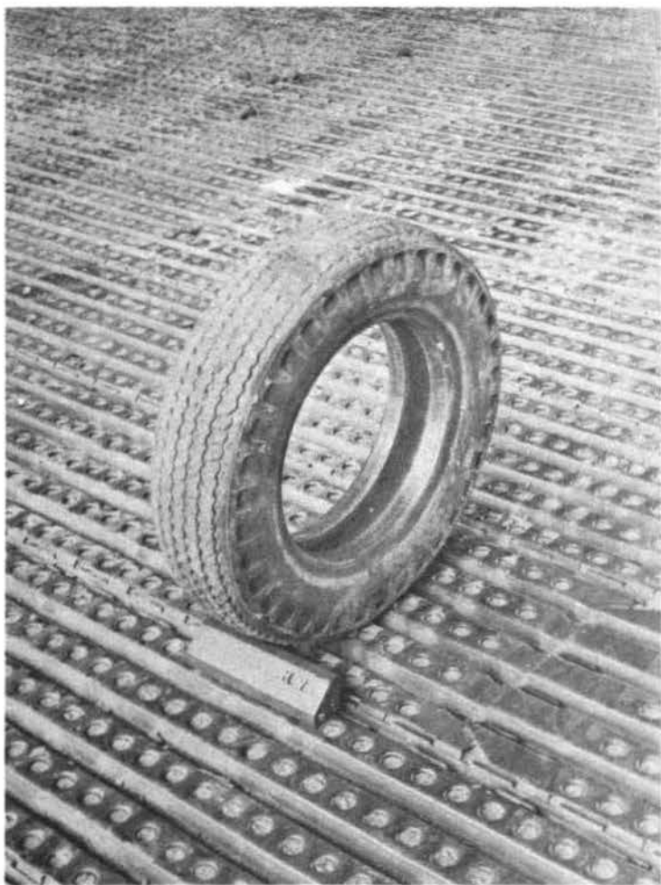
Fig. 1. Appearance of tire after test on M7 mat
