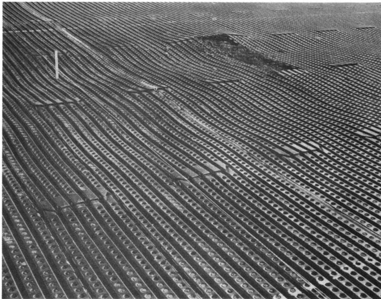
Appearance of M7 mat surface, subsection 5b after 182 coverages (the half plank was removed to permit soil sampling)
