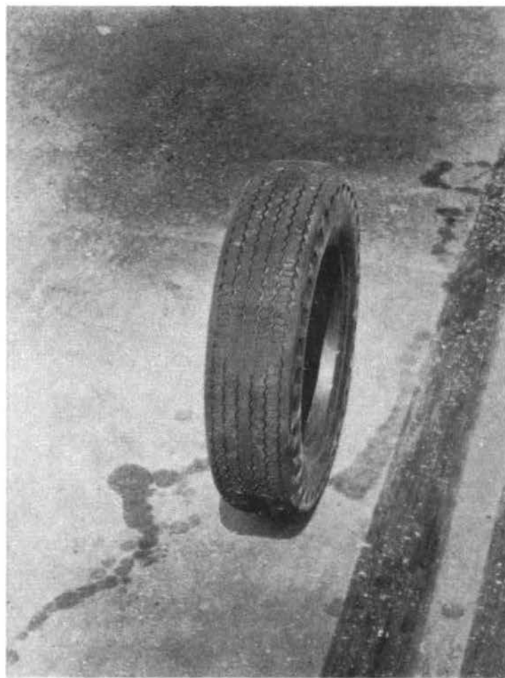
Fig. 2. Appearance of tire after test on asphalt concrete pavement
