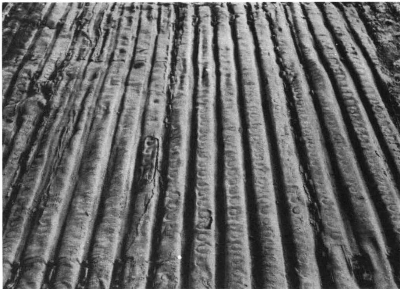
Appearance of PBS after removal of M7 mat at 1000 coverages
