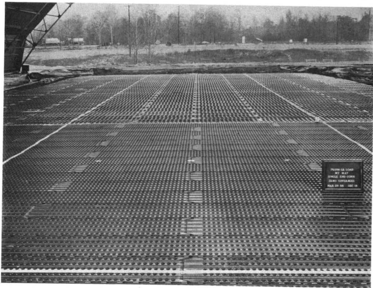
M7 and M6 mats in lane 1 before testing
