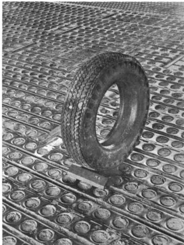
Fig. 2. Appearance of tire after test on M6 mat
