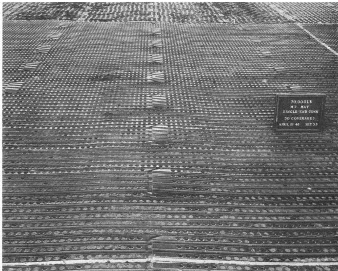
M7 mat in subsection 5b after 50 coverages
