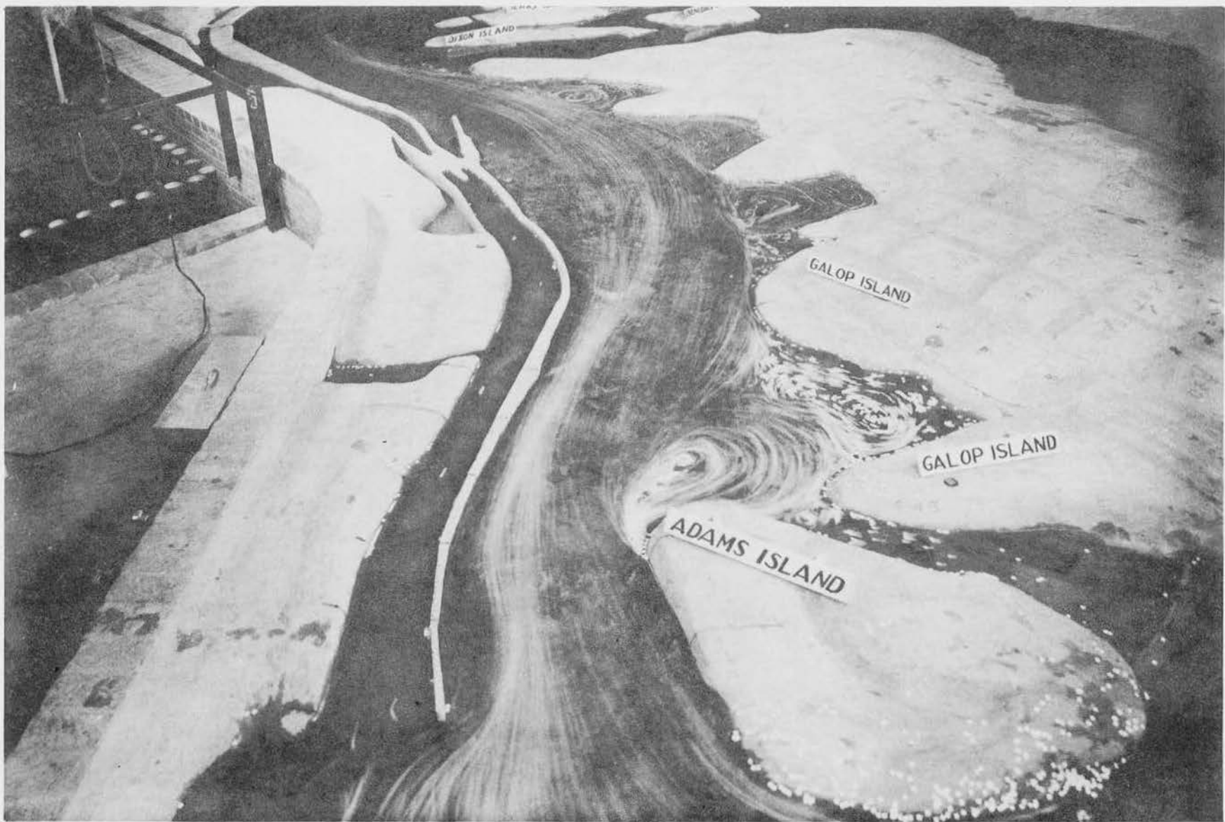
Base tests -- downstream view of Galop Island north channel
