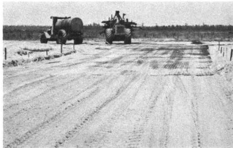
Sprinkled and natural-water areas during tracking; latter area covered with mat
