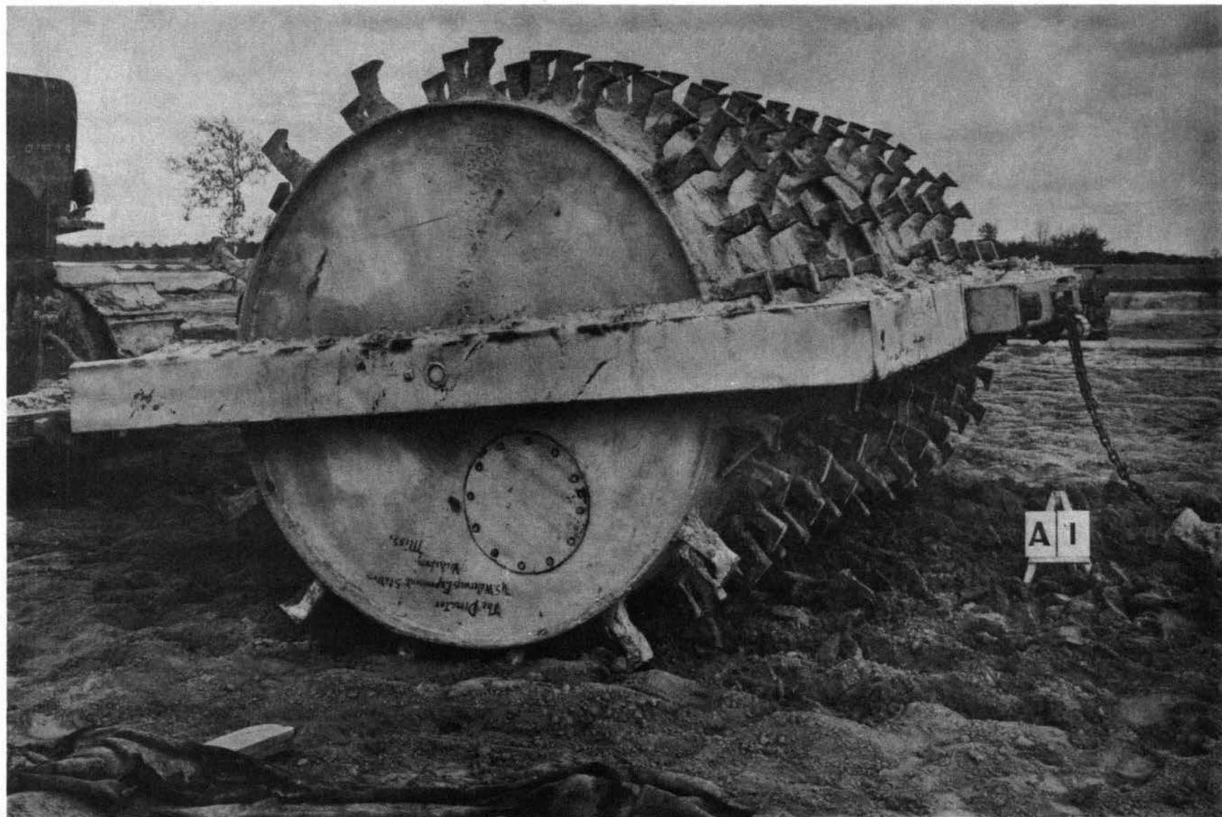
450-psi sheepsfoot roller, first pass, 6% water content
