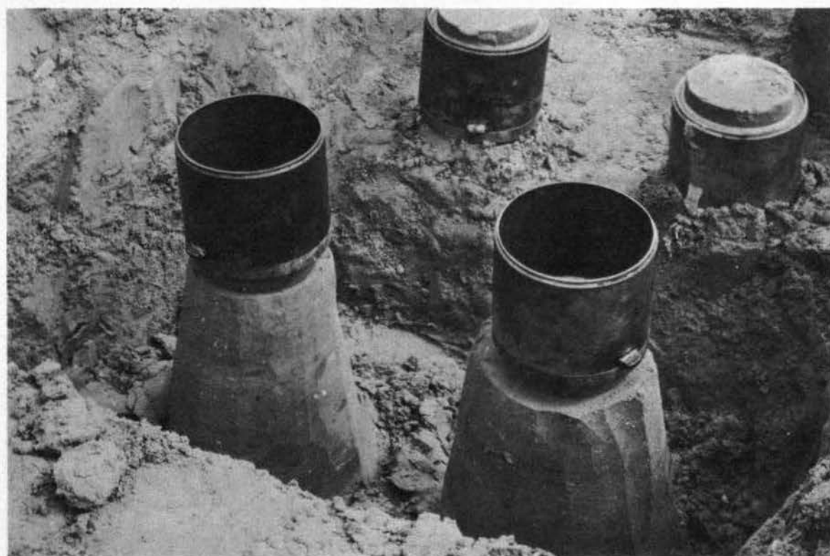
Steps in obtaining undisturbed cylinder samples in test pit
