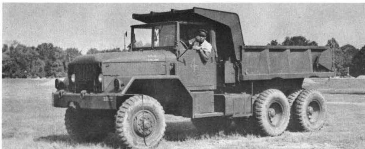
Fig. 13. M-51 test vehicle; 31,800-lb gross load, 50-psi tire pressure
