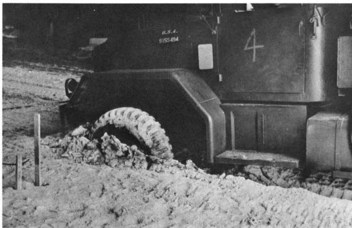
Fig. 14. Failure of test section at sta 0+00 during entry of vehicle
