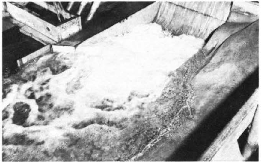
Photograph 64. Flow conditions of basin with: gates 1 through 5 open full; crest dischg, 300,000 cfs; penstocks closed; pool elev, 468.6; tailwater elev, 212.6
