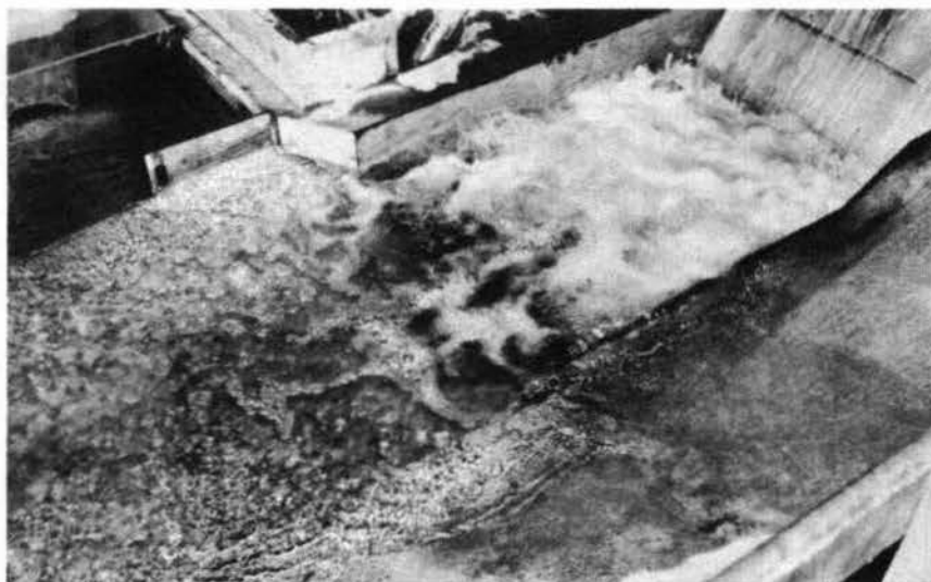
Photograph 57. Flow conditions of basin with: gates 1 through 5 open 14 ft; crest dischg, 108,000 cfs; penstock dischg, 7,000 cfs; pool elev, 466.0; tailwater elev, 179.2
