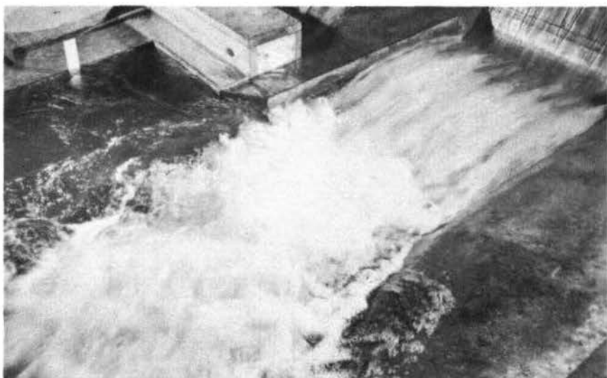
Jet action of the type 5 flip bucket
