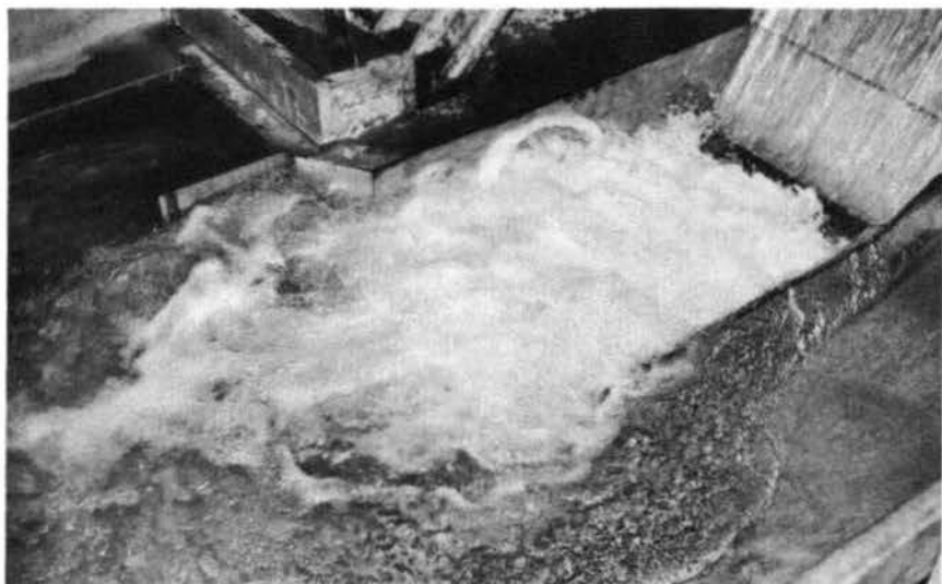
Photograph 58. Flow conditions of basin with: gates 1 through 5 open 28 ft; crest dischg, 193,000 cfs; penstock dischg, 7,000 cfs; pool elev, 466.0; tailwater elev, 196.0
