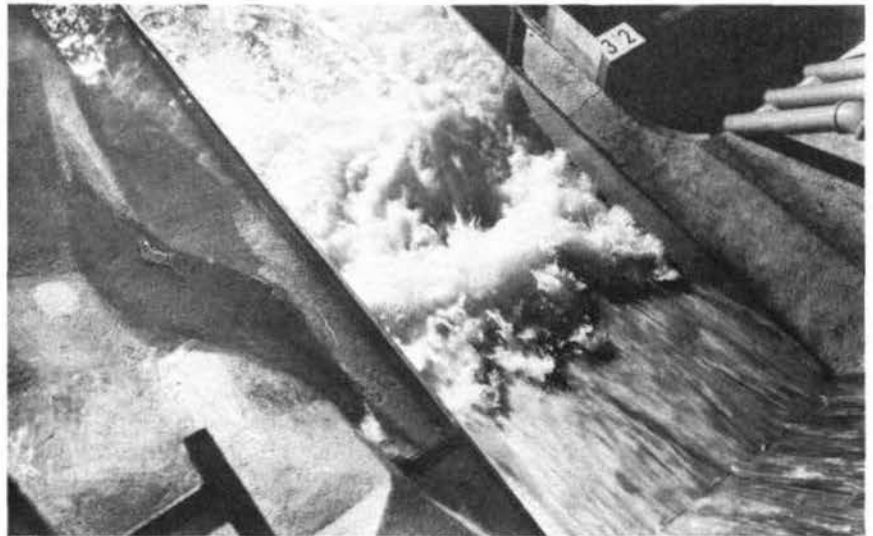
Photograph 52. Flow conditions of basin with: gates 1 through 5 open 28 ft; crest dischg, 193,000 cfs; penstock dischg, 7,000 cfs; pool elev, 466.0; tailwater elev, 196.0
