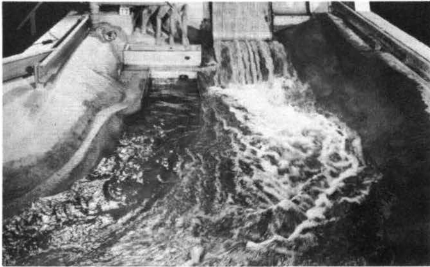
Photograph 15. Flow conditions with: gates 1 through 5 open 14 ft; crest dischg, 108,000 cfs; penstock dischg, 7,000 cfs; pool elev, 466.0; tailwater elev, 179.2
