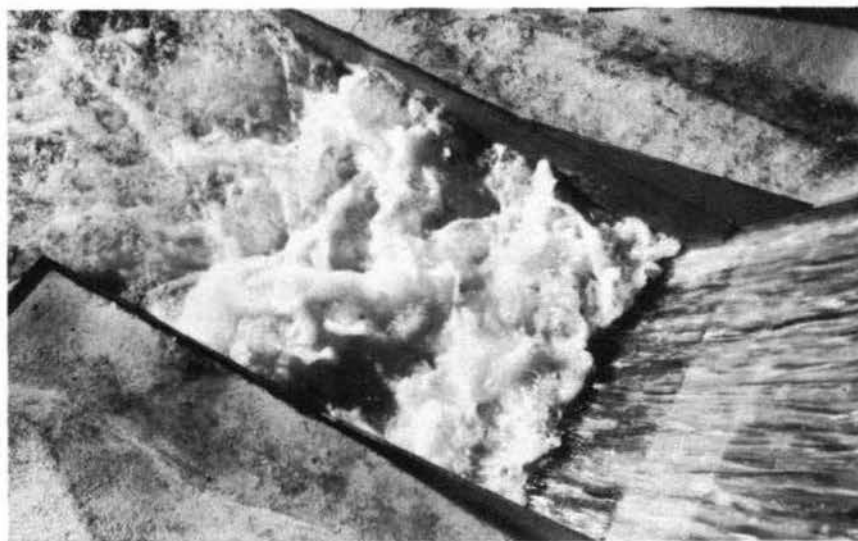
Photograph 45. Flow conditions of basin with: gates 1 through 5 open 28 ft; crest dischg, 193,000 cfs; penstock dischg, 7,000 cfs; pool elev, 466.0; tailwater elev, 196.0
