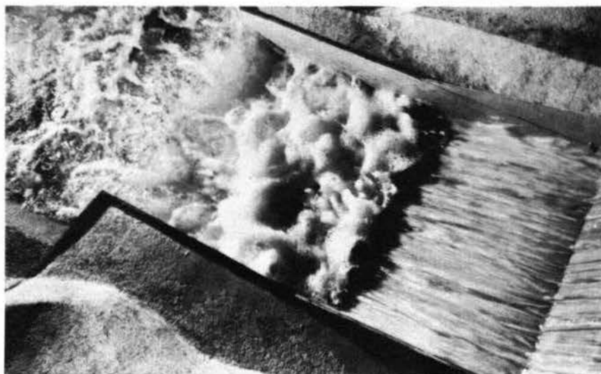
Photograph 42. Flow conditions of basin with: gates 1 through 5 open 28 ft; crest dischg, 193,000 cfs; penstock dischg, 7,000 cfs; pool elev, 466.0; tailwater elev, 196.0
