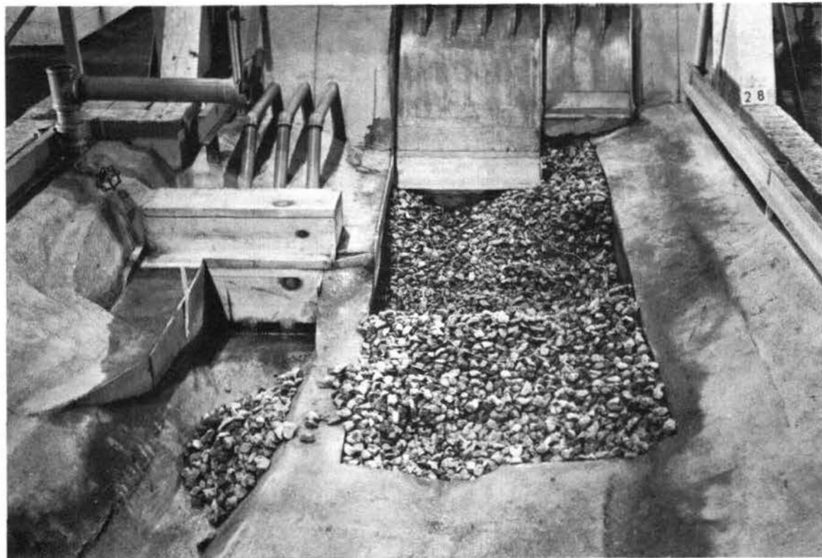
Photograph 14. View of bed downstream from original flip bucket after one-hour scour. Spillway gates 1 through 5 open 14 ft; crest dischg, 108,000 cfs; penstock dischg, 7,000 cfs; pool elev, 466.0; tailwater elev, 179.2
