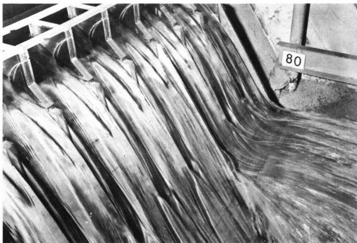
Photograph 68. Flow conditions along type B center training wall. Gates 1 through 8 open full. Crest dischg, 567,000 cfs; pool elev, 473.8
