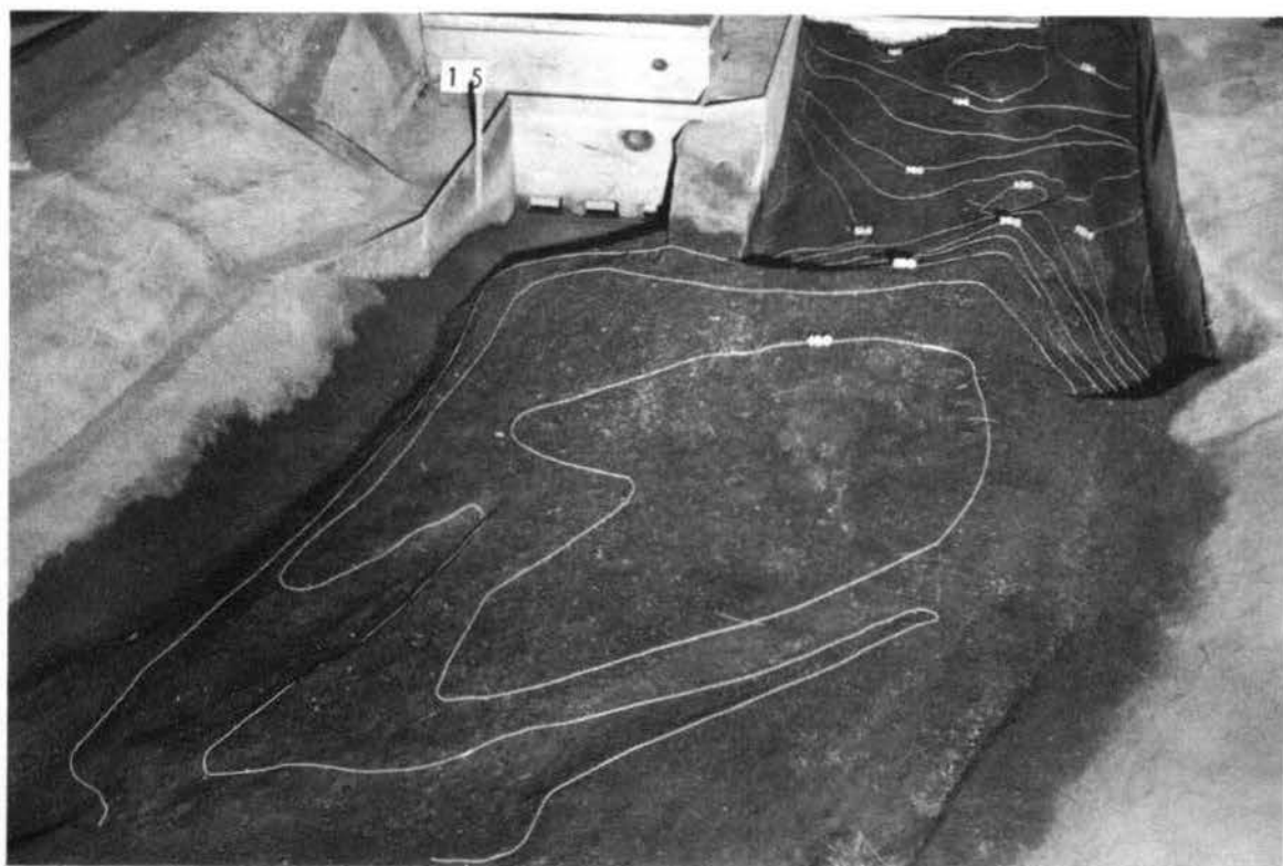
Fig. 4. Bed downstream from flip bucket after 1-hour scour, Model A. Discharge, 115,000 cfs; pool elev, 466.0
