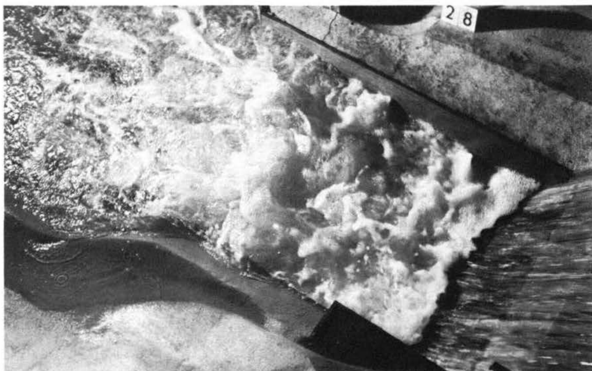
Photograph 48. Gates 1 through 5 open 28 ft; crest dischg, 193,000 cfs; penstock dischg, 7,000 cfs; pool elev, 466.0; tailwater elev, 196.0
