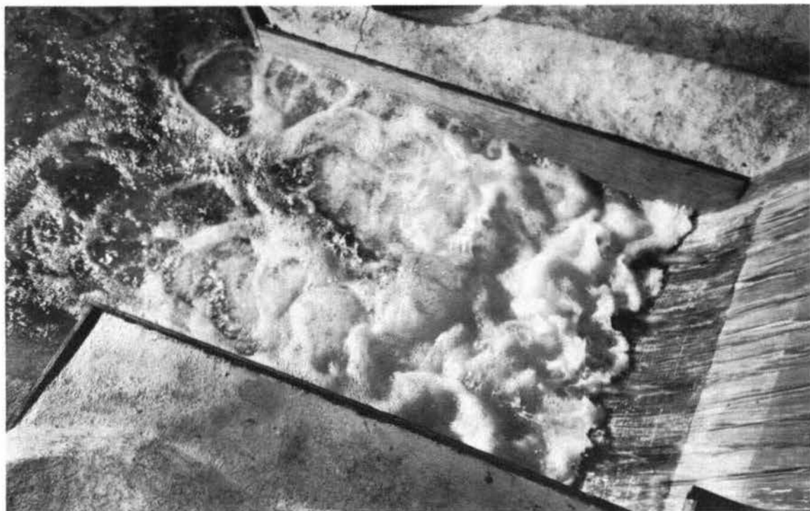
Photograph 34. Gates 1 through 5 open 14 ft; crest dischg, 108,000 cfs; penstock dischg, 7,000 cfs; pool elev, 466.0; tailwater elev, 179.2
