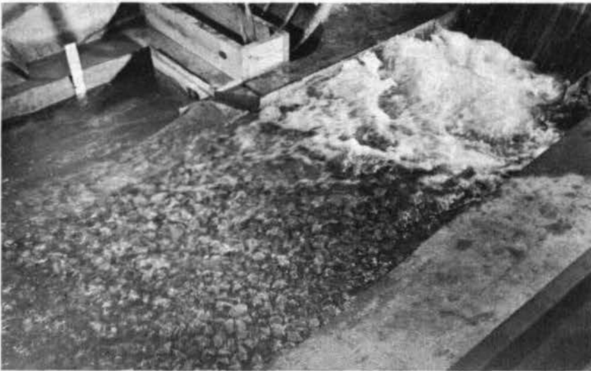
Photograph 27. Jet action of bucket. Gates 1 through 5 open 14 ft; crest dischg, 108,000 cfs; penstock dischg, 7,000 cfs; pool elev, 466.0; tailwater elev, 179.2
