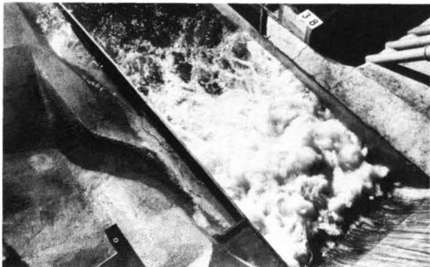
Photograph 54. Flow conditions of basin with: gates 1 through 5 open 14 ft; crest dischg, 108,000 cfs; penstock dischg, 7,000 cfs; pool elev, 466.0; tailwater elev, 179.2
