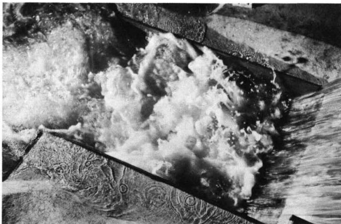
Photograph 37. Stilling-basin action in the type 2 stilling basin
