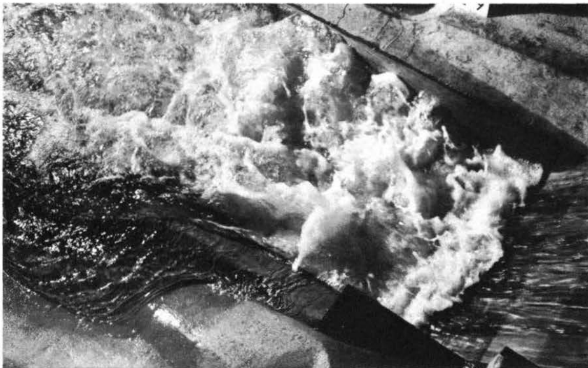
Photograph 49. Gates 1 through 5 open full; crest dischg, 300,000 cfs; penstocks closed; pool elev, 468.6; tailwater elev, 212.6
