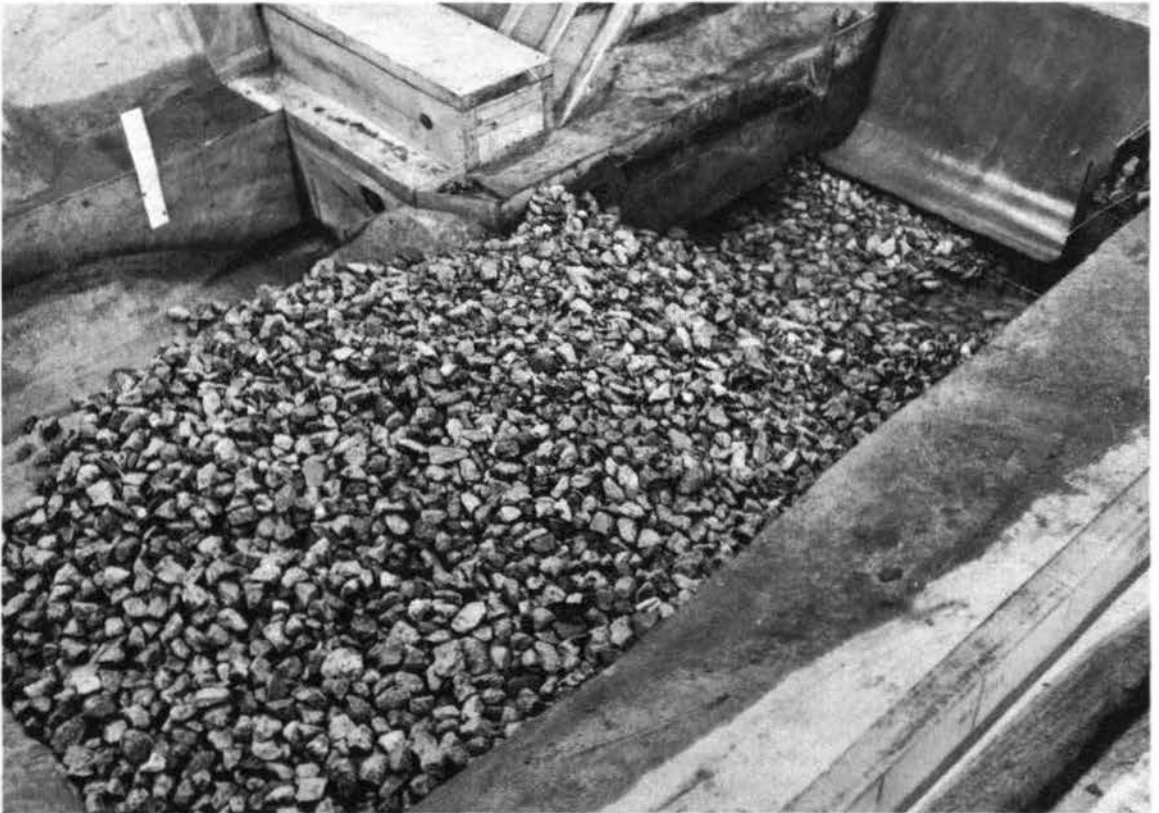
Fig. 7. View of the bed downstream of the type 6 flip bucket, Model A. Scour after successive discharges of 115,000, 200,000 and 300,000 cfs for 15 minutes of model operation
