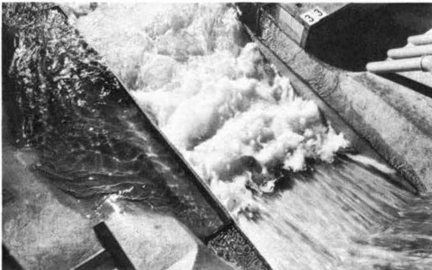
Photograph 53. Flow conditions of basin with: gates 1 through 5 open full; crest dischg, 300,000 cfs; penstocks closed; pool elev, 468.6; tailwater elev, 212.6
