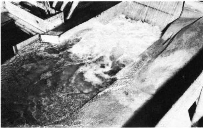
Photograph 62. Flow conditions of basin with: gates 1 through 5 open 14 ft; crest dischg, 108,000 cfs; penstock dischg, 7,000 cfs; pool elev, 466.0; tailwater elev, 179.2
