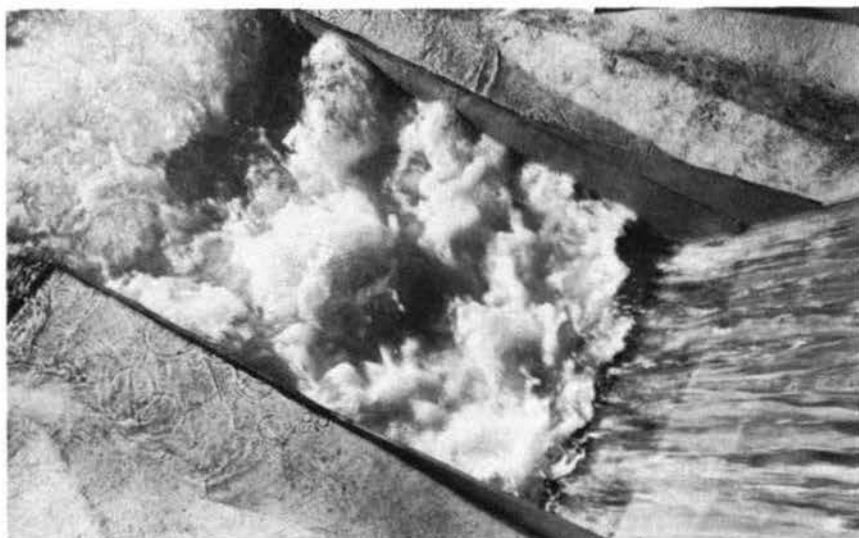
Stilling-basin action in the type 9 stilling basin
