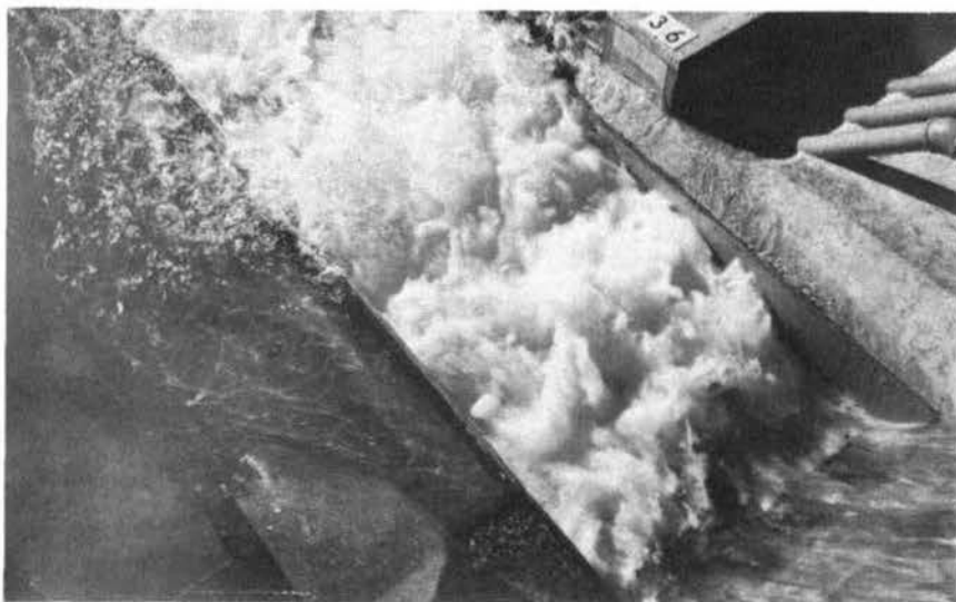
Stilling-basin action in the type 12 stilling basin
