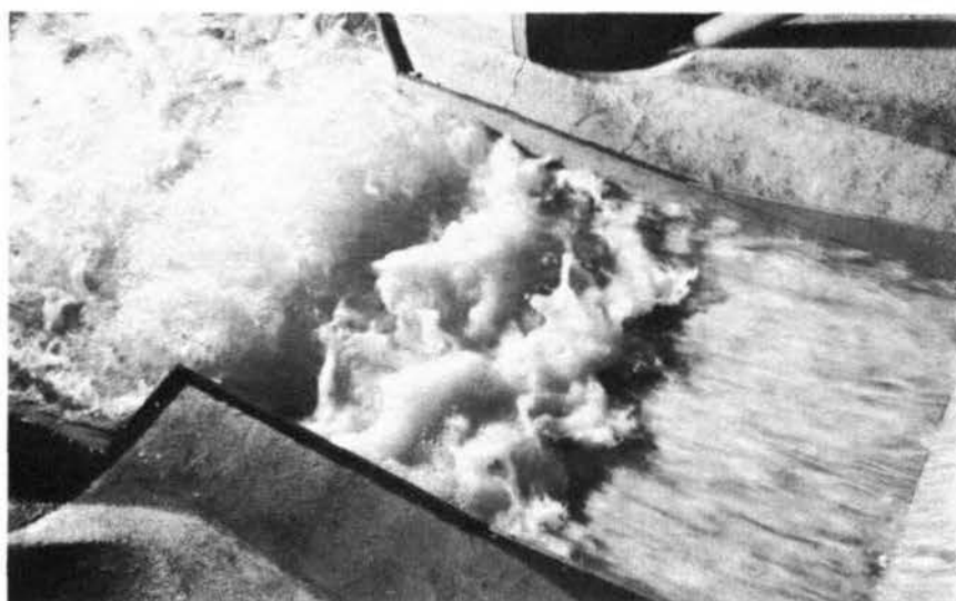
Photograph 42. Flow conditions of basin with: gates 1 through 5 open 28 ft; crest dischg, 193,000 cfs; penstock dischg, 7,000 cfs; pool elev, 466.0; tailwater elev, 196.0
