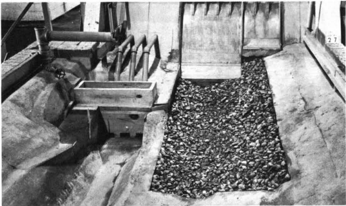
Photograph 13. View of bed downstream from original flip bucket before scour test. Note large gravel as a bed material replacing pea gravel
