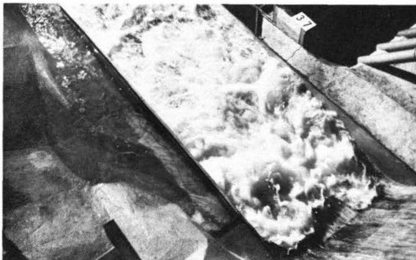
Photograph 55. Flow conditions of basin with: gates 1 through 5 open 28 ft; crest dischg, 193,000 cfs; penstock dischg, 7,000 cfs; pool elev, 466.0; tailwater elev, 196.0
