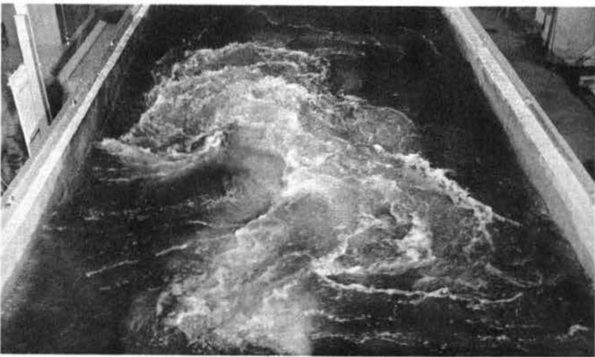
Fig. 4. Ten-foot-high end sill of modification D maintained tailwater depths capable of containing the excess energy of the conduit discharge (3500 cfs) within the stilling basin at all times
