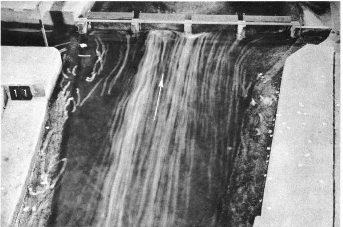
Photograph 7. Original design: Surface currents approaching Woonsocket Falls Dam, discharge 30,000 cfs. Note concentration of flow toward center bays
