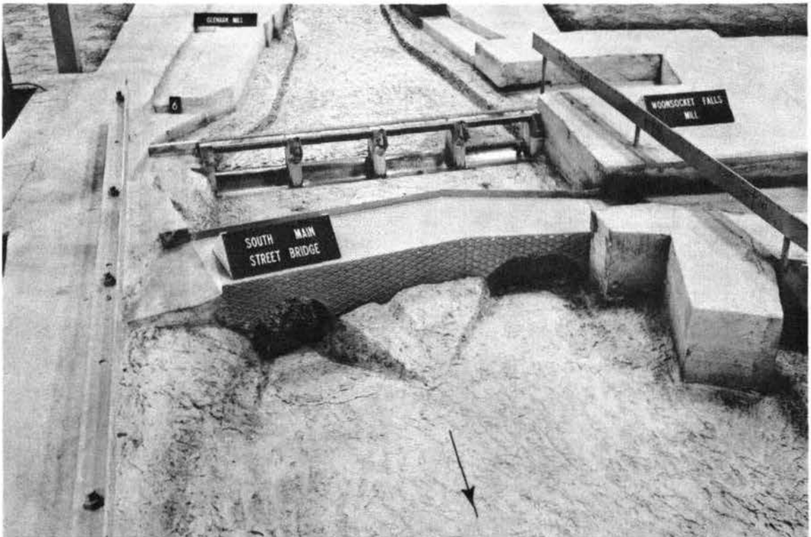
Photograph 4. Original design: Rock excavation below arches of South Main Street bridge
