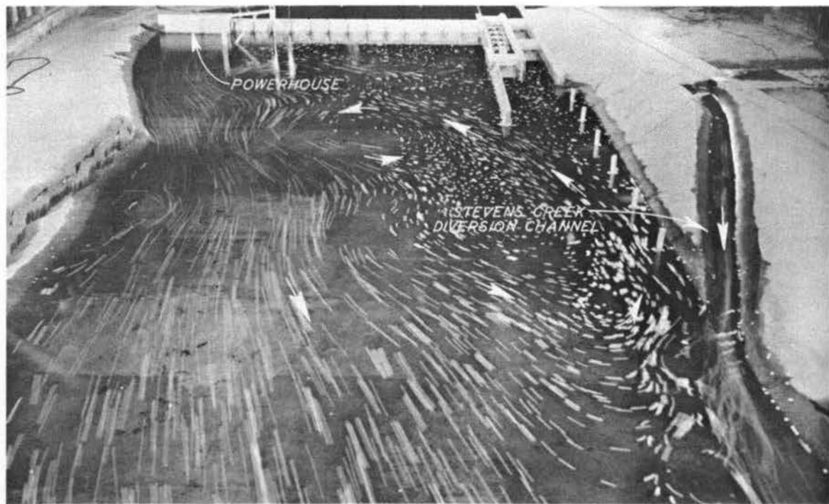
Photograph 26. Plan B: effects of Stevens Creek diversion channel outlet at sta 41+10 on surface currents with powerhouse in operation. Powerhouse discharge, 65,000 cfs; Stevens Creek discharge, 4,500 cfs
