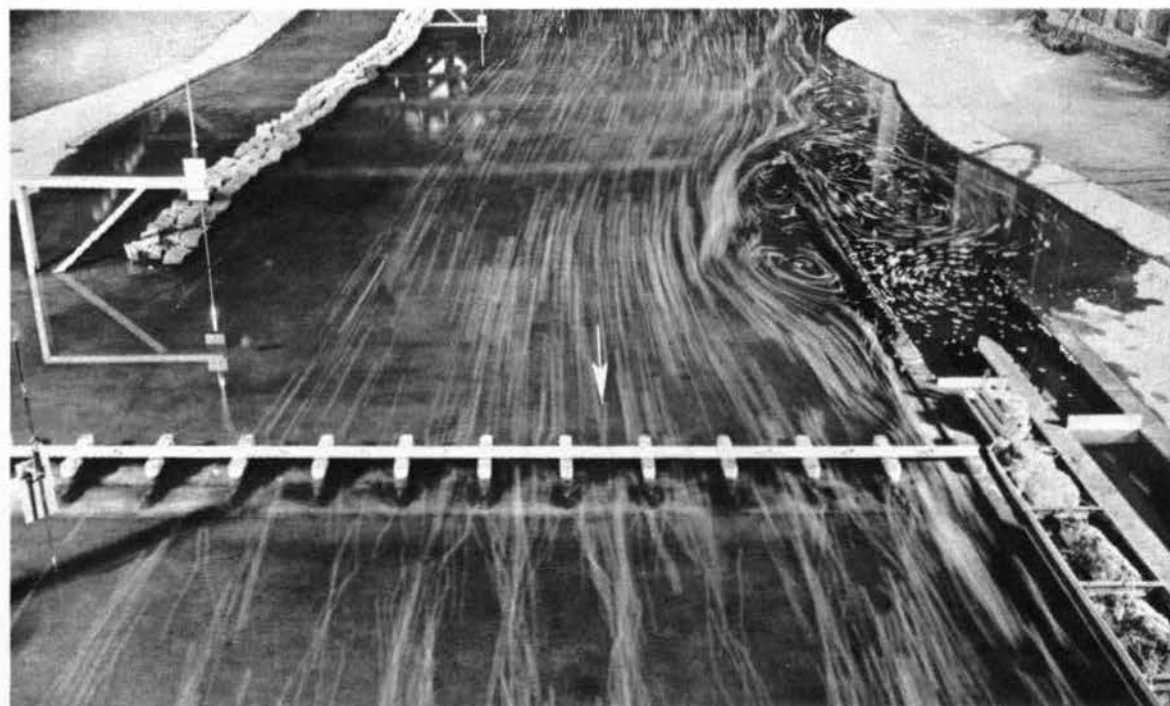
Photograph 4. Plan A: surface currents in upper lock approach with no ports in upper guard wall. Discharge, 640,000 cfs
