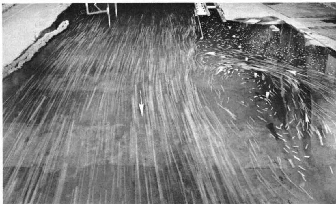
Photograph 10. Plan A: surface currents in lower lock approach. Discharge, 640,000 cfs
