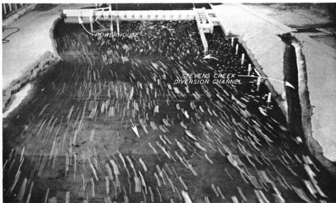
Photograph 14. Plan B: surface currents in lower lock approach with flow divided evenly between powerhouse and dam and no flow in Stevens Creek diversion channel. Powerhouse discharge, 50,000 cfs; dam discharge, 50,000 cfs
