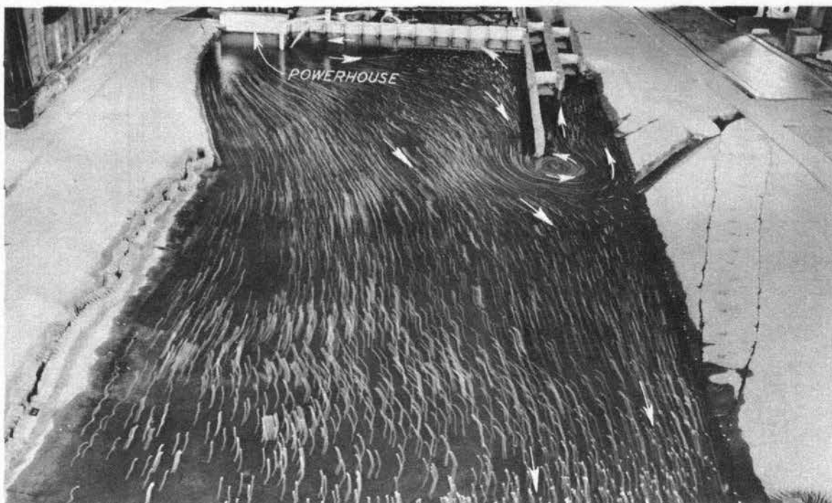
Photograph 19. Plan B: flow conditions in lower approach 2 minutes after powerhouse discharge was increased from 0 to 65,000 cfs. Note strong eddy at end of lower guard wall
