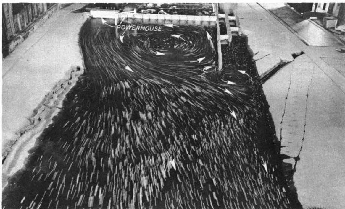
Photograph 20. Plan B: flow conditions in lower approach 7 minutes after powerhouse discharge was increased from 0 to 65,000 cfs with no flow over dam. Note change in size and intensity of eddy at end of lower guard wall from that shown on photograph 19
