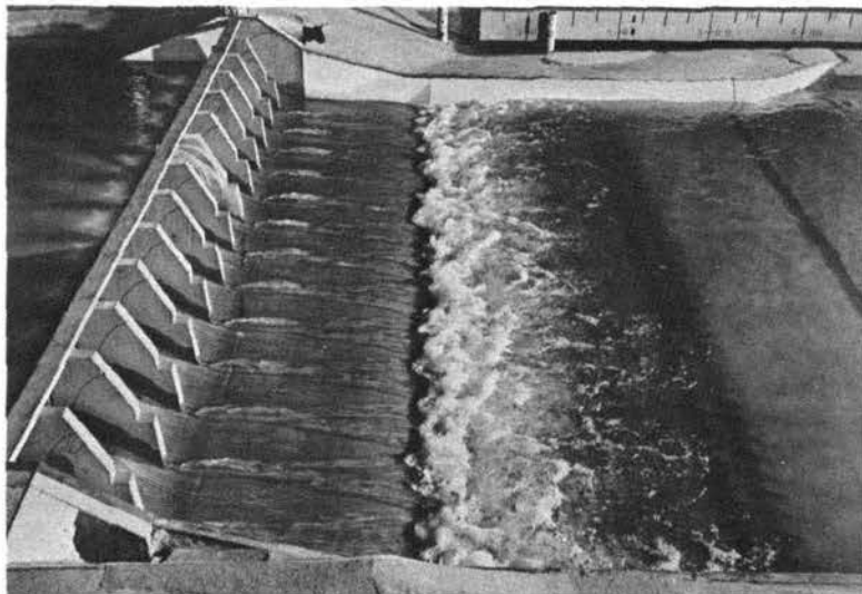
Fig. 10. Stilling action, adopted design. Discharge, 100,000 cfs
