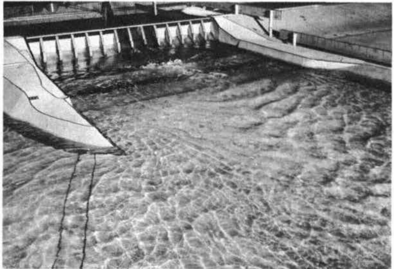
Fig. 13. Stilling action, adopted design. Pool elevation, 1210.0
