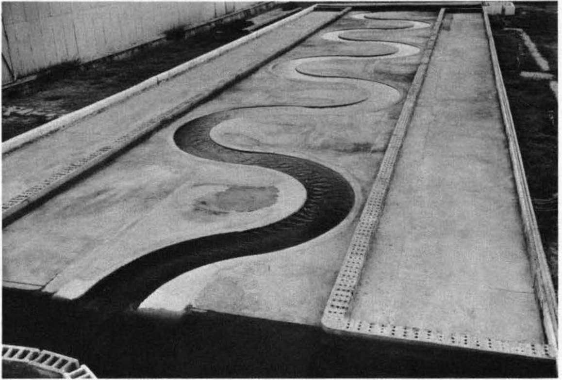
Fig. 2. Floodway width was varied by means of brick walls; here, it is 16 ft
