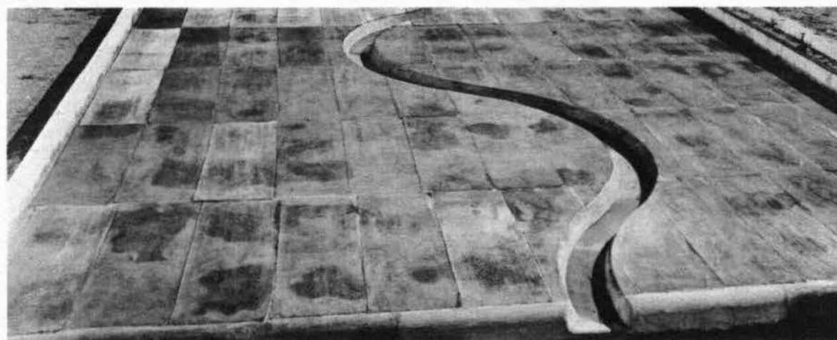
Expanded metal with long dimension parallel to flow, n = 0.025
