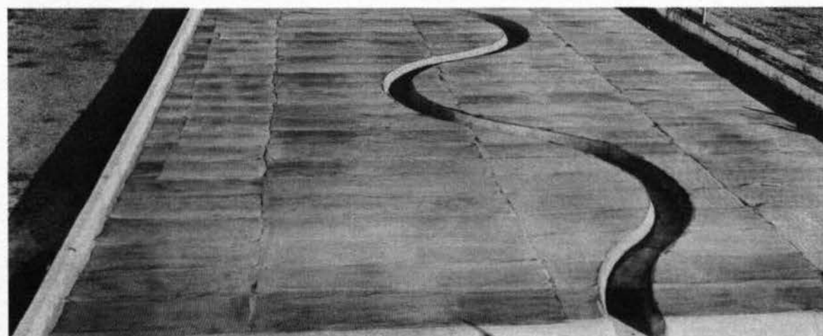
Expanded metal with long dimension normal to flow, n = 0.035
