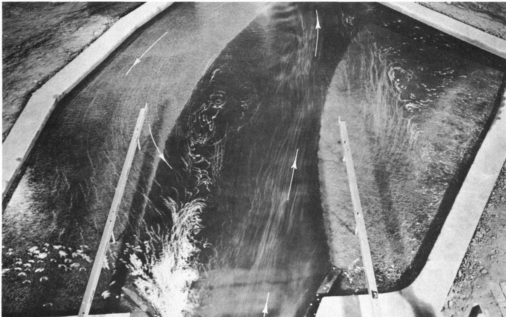
Photograph 6. Original design: surface currents below transition. Note concentration of flow towards right. Compare with photograph 4. Discharge, 20,000 cfs; tailwater elevation, 15.4 ft msl
