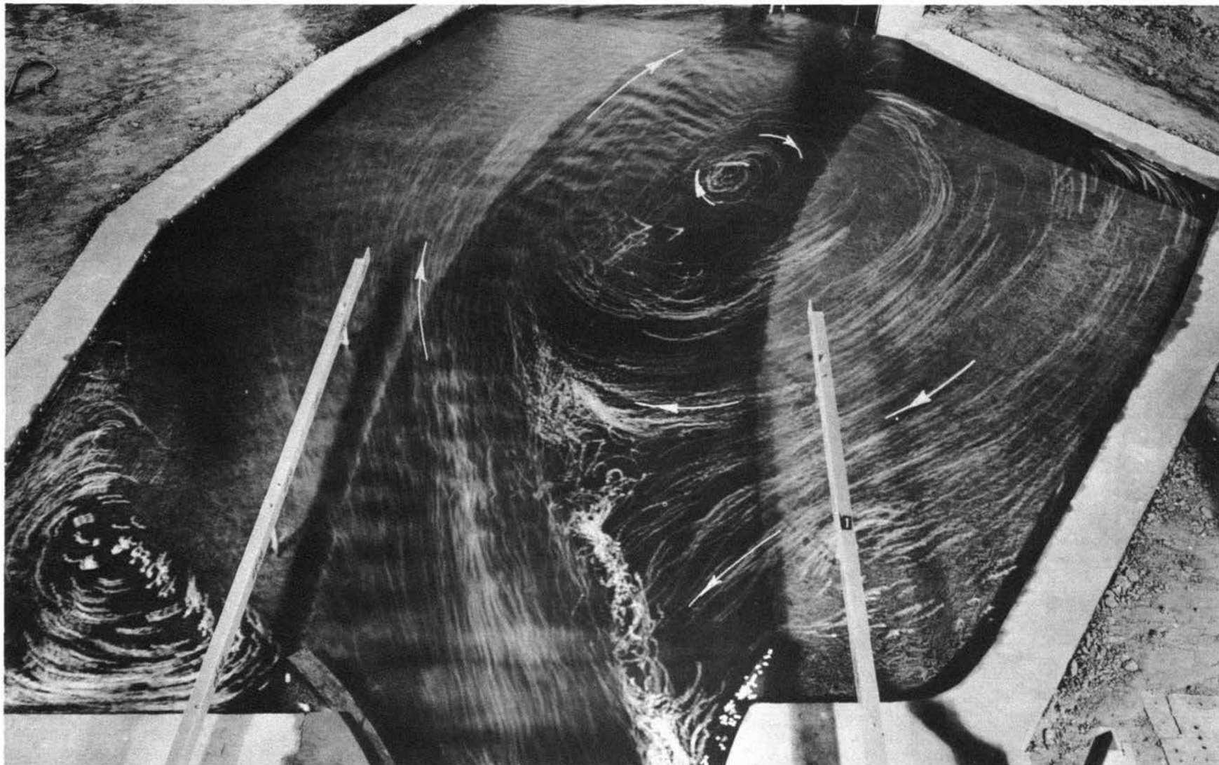
Photograph 4. Original design: surface currents below transition. Discharge, 20,000 cfs; tailwater elevation, 19.4 ft msl
