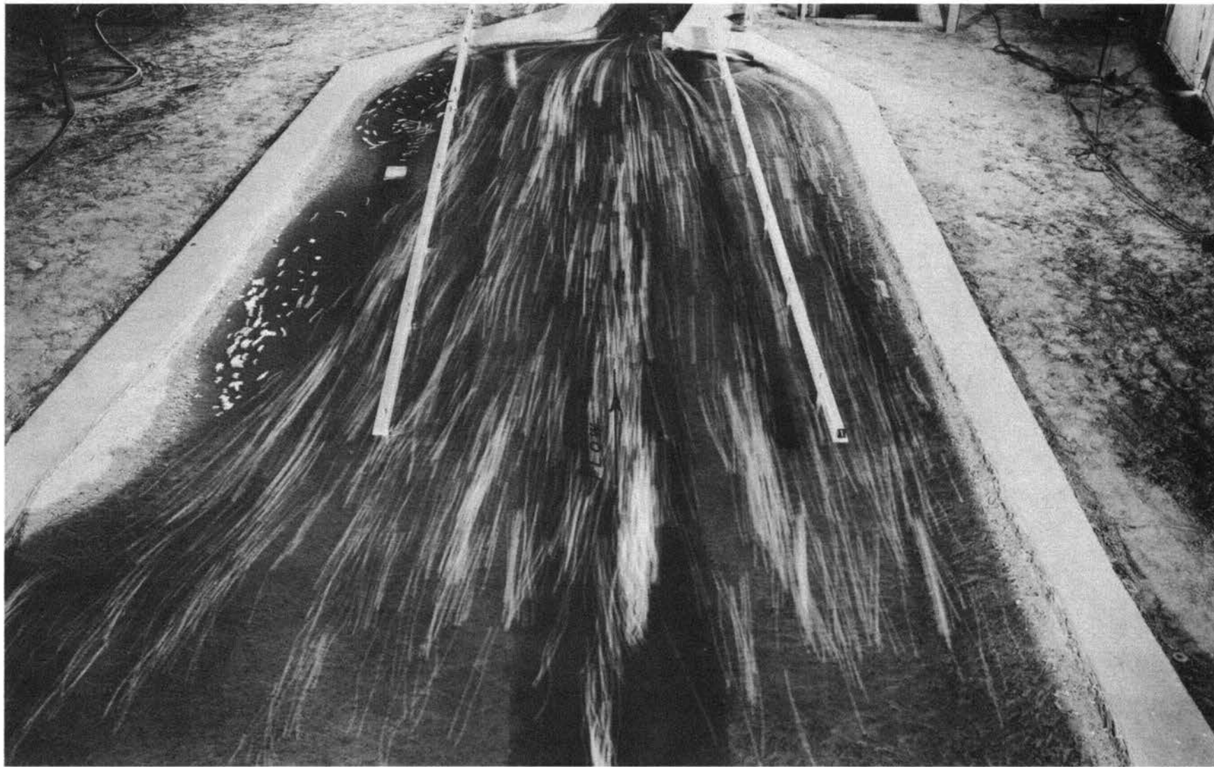
Photograph 1. Original design: surface currents in reach above control section. Discharge, 20,000 cfs; tailwater elevation, 19.4 ft msl
