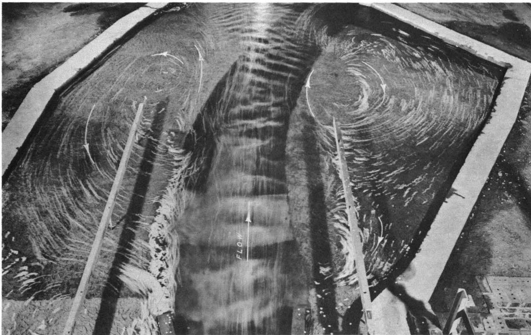
Photograph 11. Plan C: surface currents below transition. Discharge, 20,000 cfs; tailwater elevation, 19.4 ft msl
