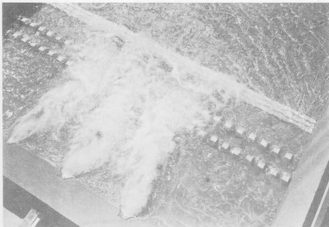
PHOTOGRAPH 14. Three type A-1 sluices in operation Discharge 5,080 cfs, pool elev 765.0, tailwater elev 707.0
