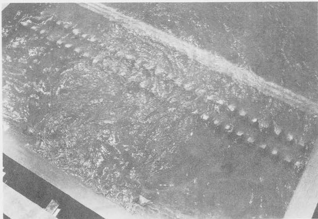
PHOTOGRAPH 15. Nine type A-1 sluices in operation Discharge 14,040 cfs, pool elev 765.0, tailwater elev 718.9
