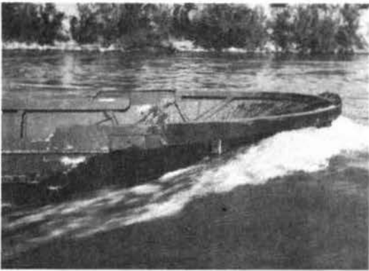
Two-ponton M4 raft -- normal spacing Pontons with 10-in. freeboard in still water being towed about 8 fps
