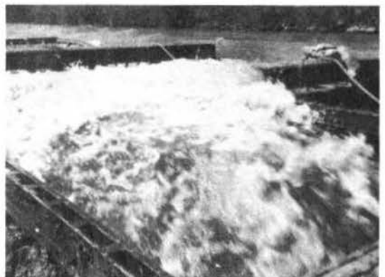
Two-ponton M4 raft -- normal spacing Pontons with 14-in. freeboard in still water being towed about 12 fps
