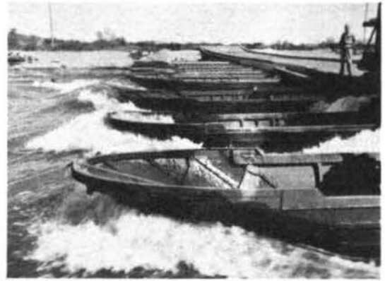
55-ton load on center line Current of approximately 10 fps Side freeboard, still water, 11 in.
