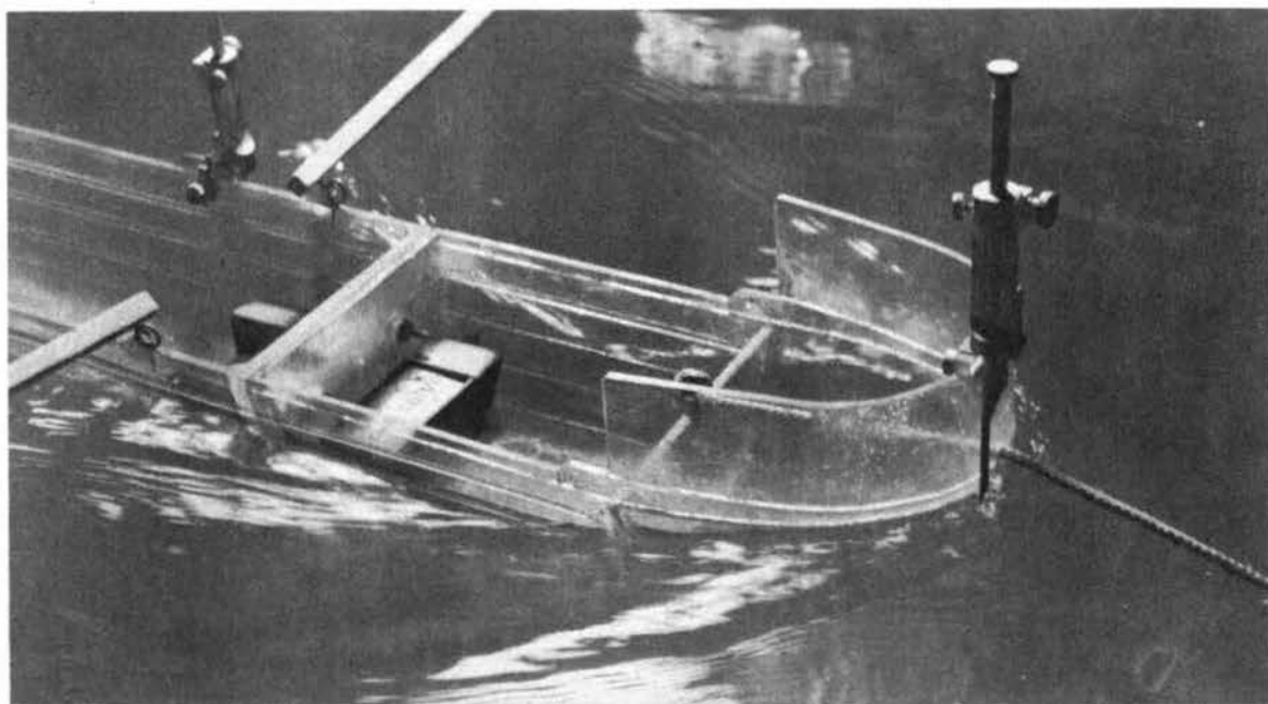
Figure 5. Flow conditions for single M4 ponton Freeboards for velocity of 10.8 fps and 14-in. loading Bow 10.0 in. Side 10.5 in.
