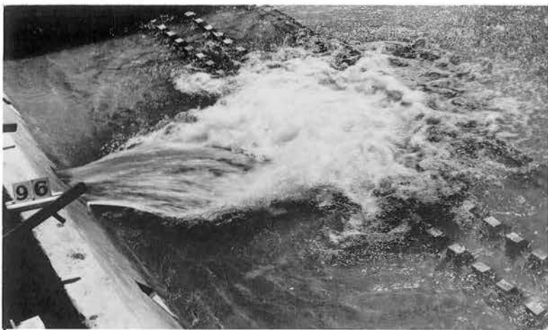
c. Discharge 2520 cfs Pool elev 987.5 Tailwater elev 913.3
