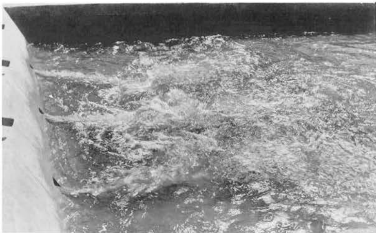
a. Discharge 5,630 cfs Pool elev 962.5 Tailwater elev 916.8
