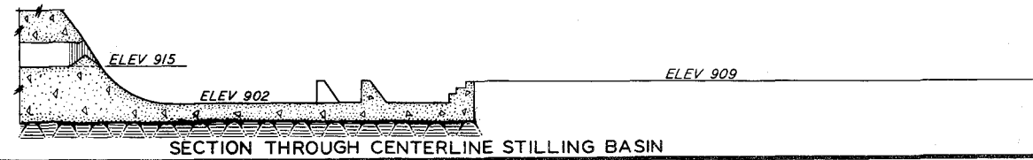
MODEL STUDY OF SLUICES FALL RIVER DAM FALL RIVER, KANSAS SCOUR PATTERN
