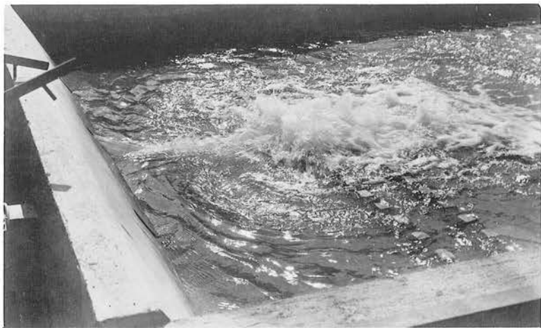
c. Discharge 2400 cfs Pool elev 987.5 Tailwater elev 912.8
