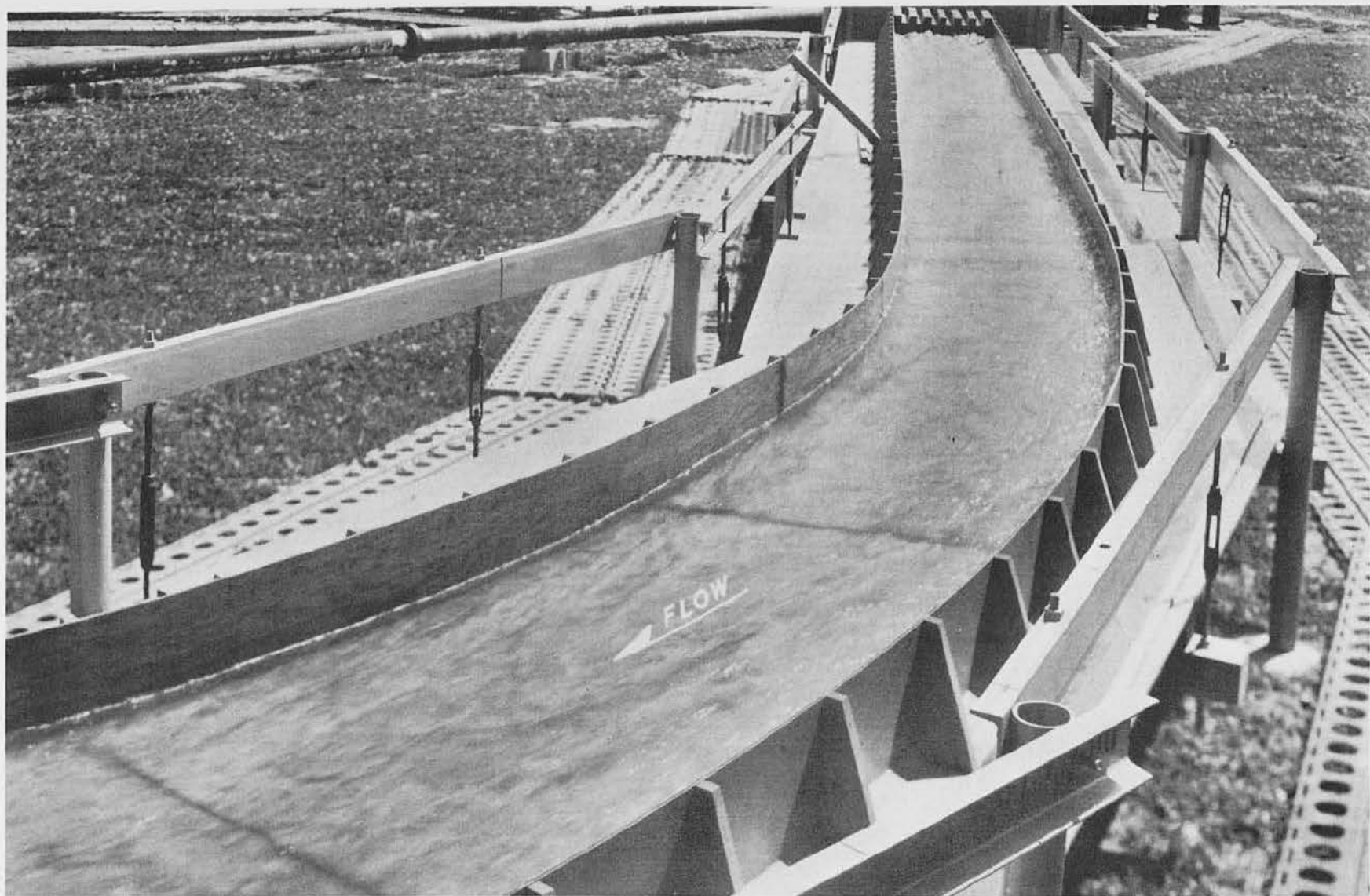
Original design, main channel. Station 63+00 to station 55+00 Discharge 8,200 cfs
