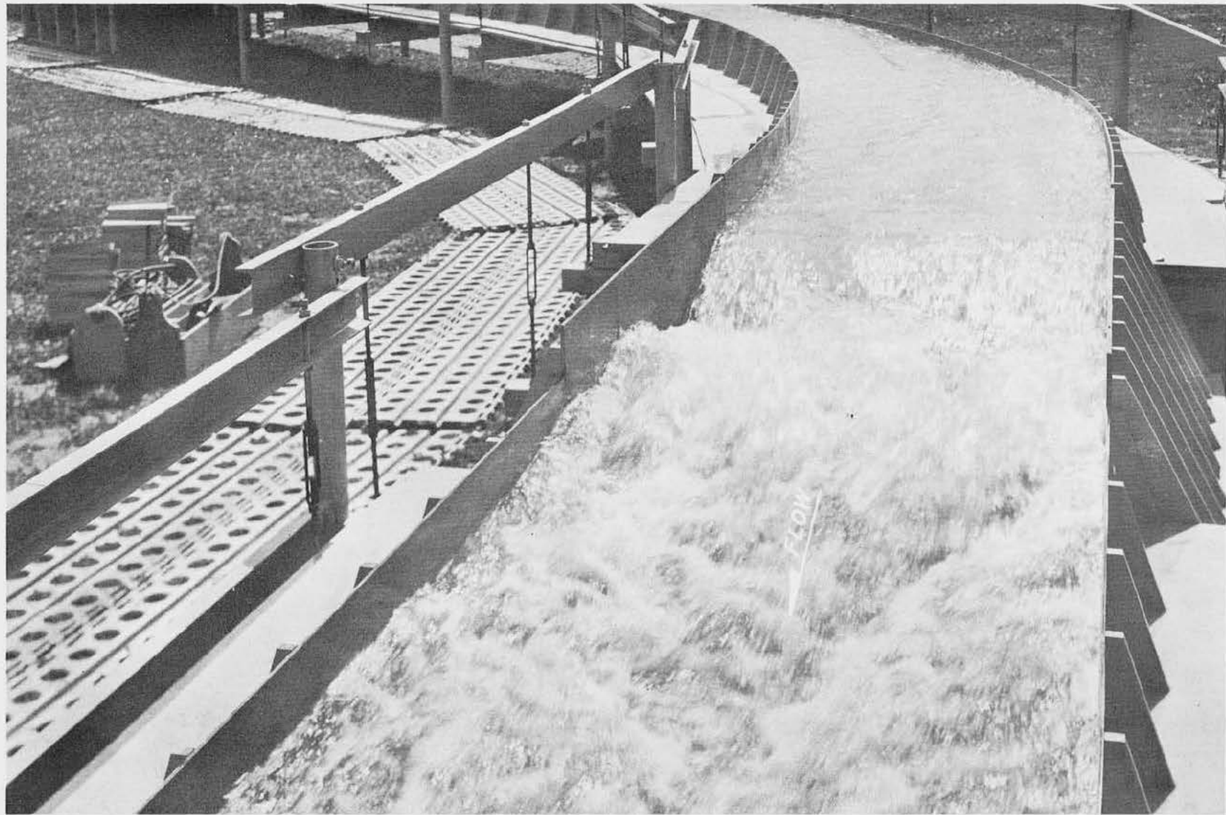
Original design, stilling basin Discharge 8,200 cfs
