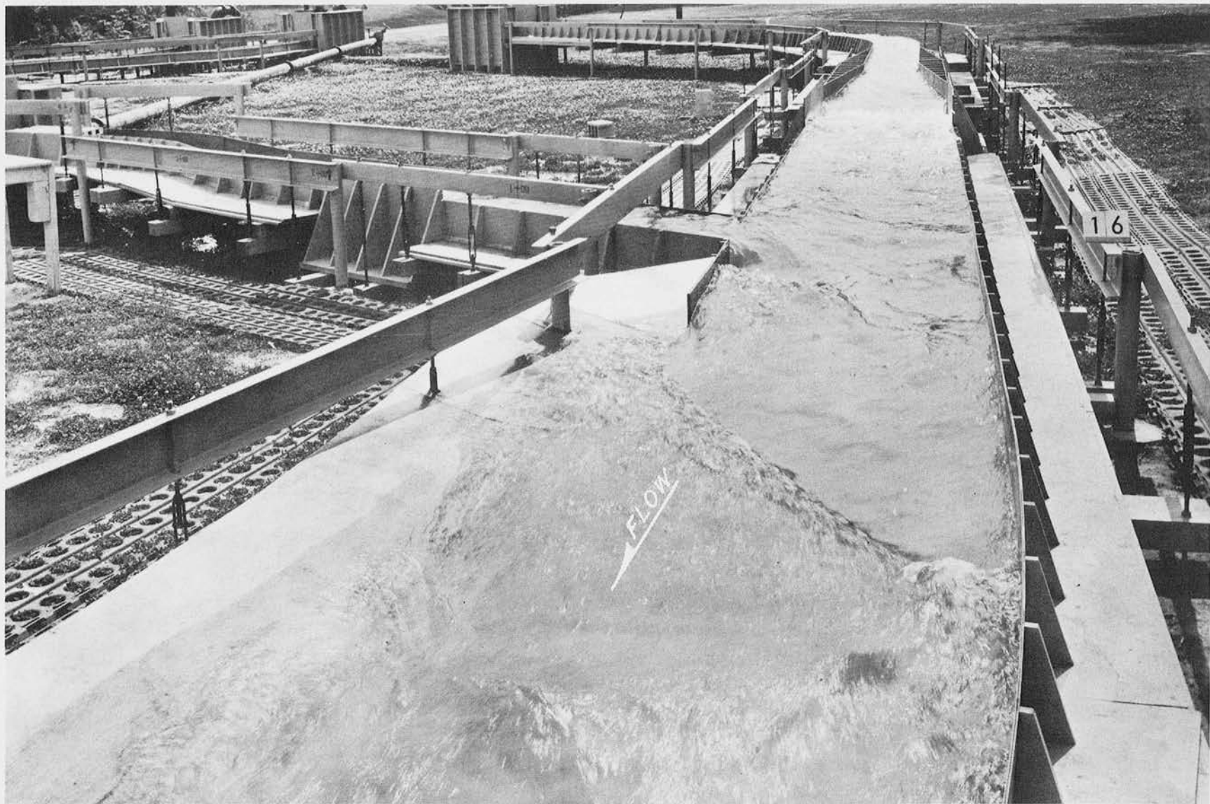
Original design, junction of Tophet Brook with Plan 3 channel Discharge: Tophet Brook 2,000 cfs; Hoosic River 13,000 cfs
