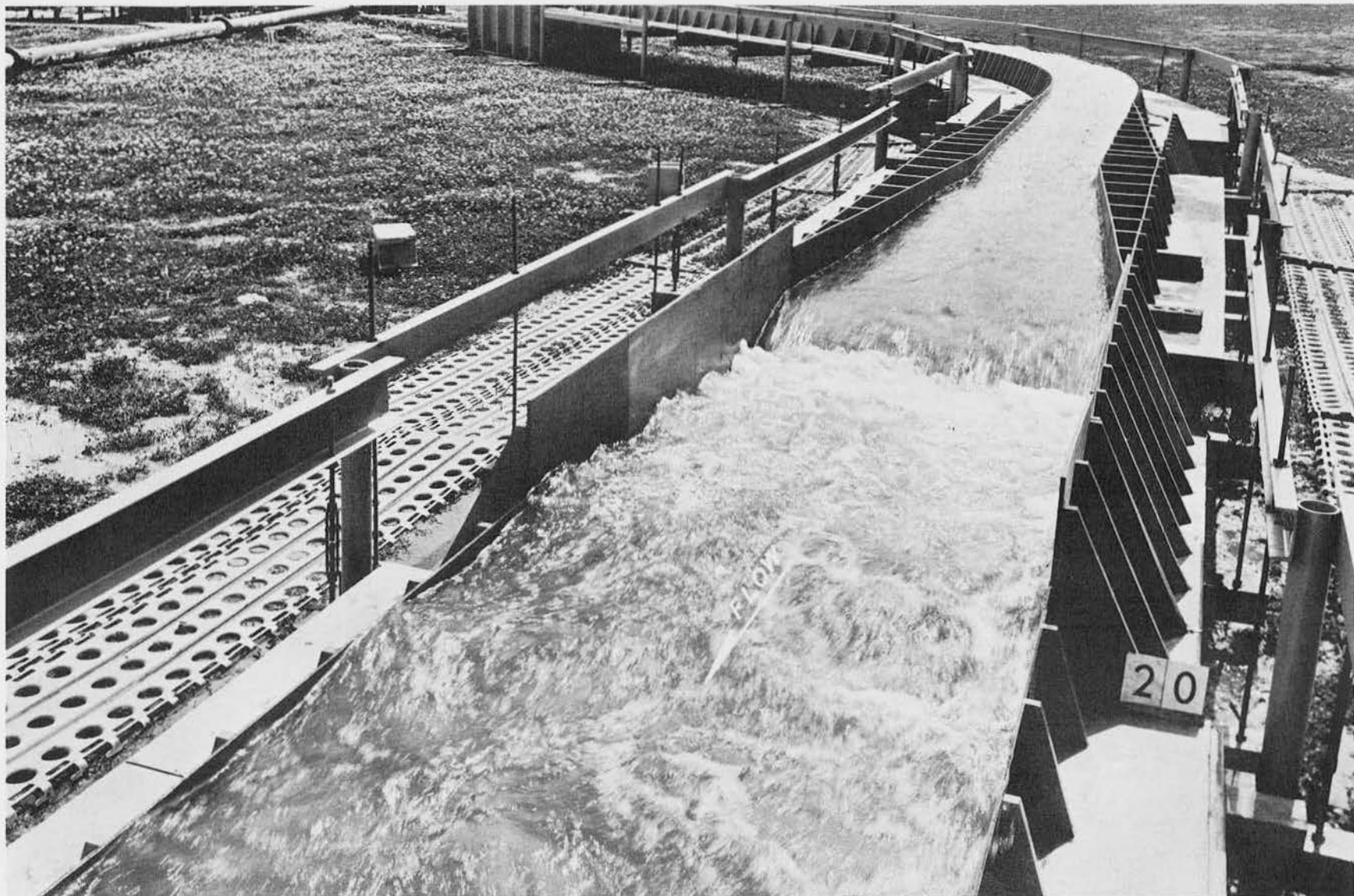
Plan 3 stilling basin Discharge 13,000 cfs
