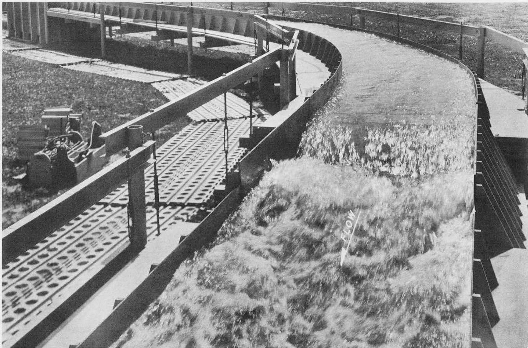
Original design, stilling basin Discharge 13,000 cfs
