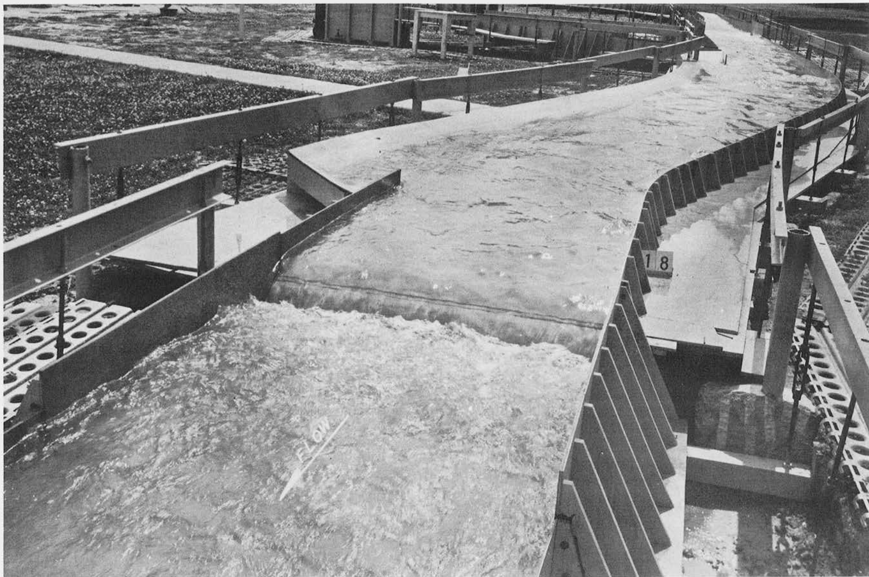
Plan 3 design, overflow weir lower end of model Discharge: Tophet Brook 2,000 cfs; Hoosic River 8,200 cfs
