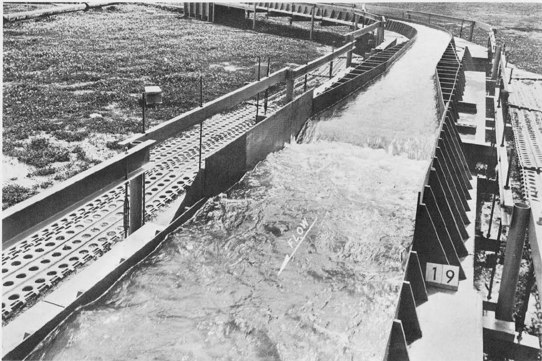
Plan 3 stilling basin Discharge 8,200 cfs
