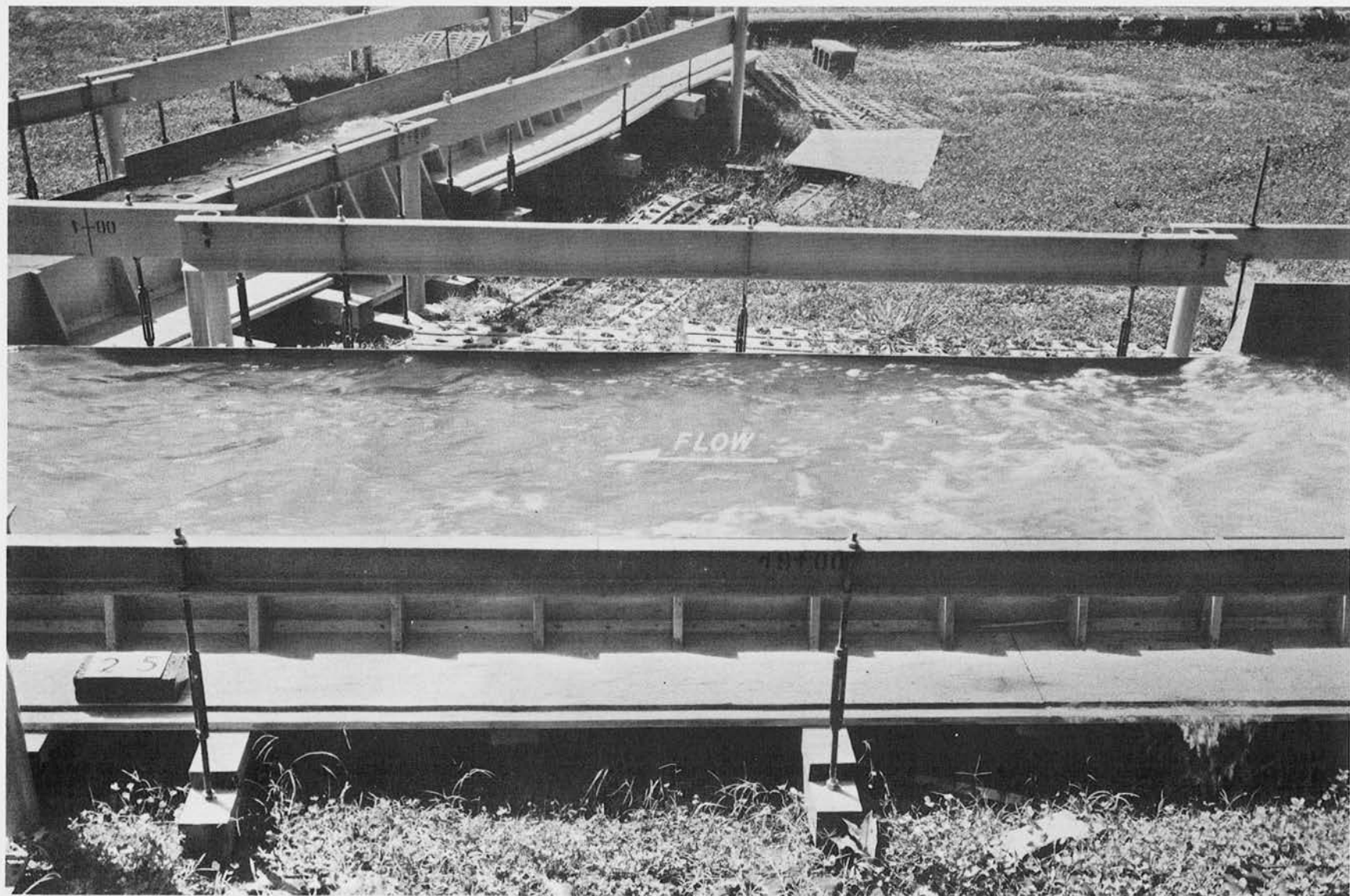
Plan 3 design, main channel. Station 47+50 to station 50+00 Discharge 13,000 cfs
