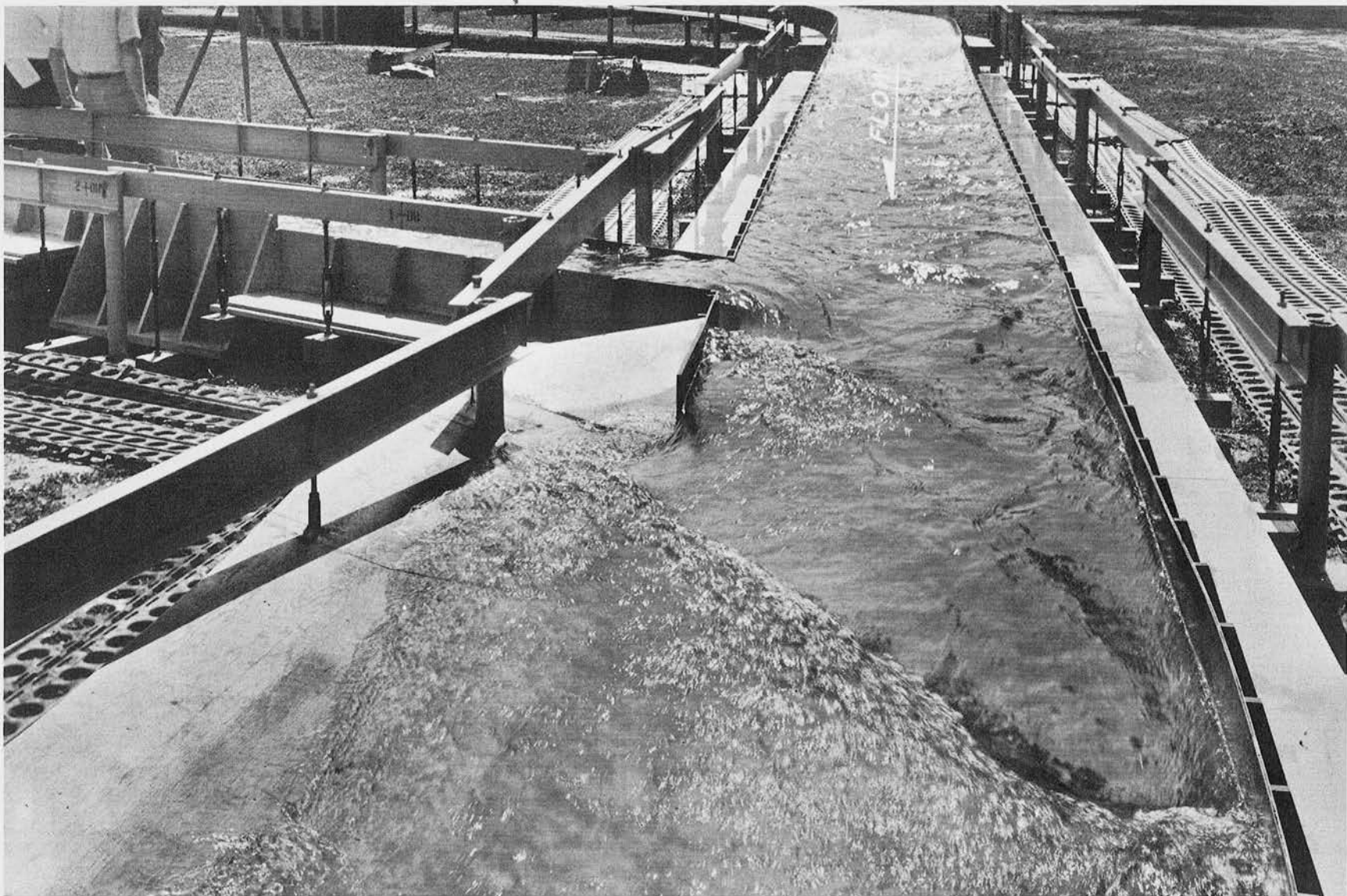
Original design, junction Tophet Brook Discharge: Hoosic River 13,000 cfs; Tophet Brook 2,000 cfs
