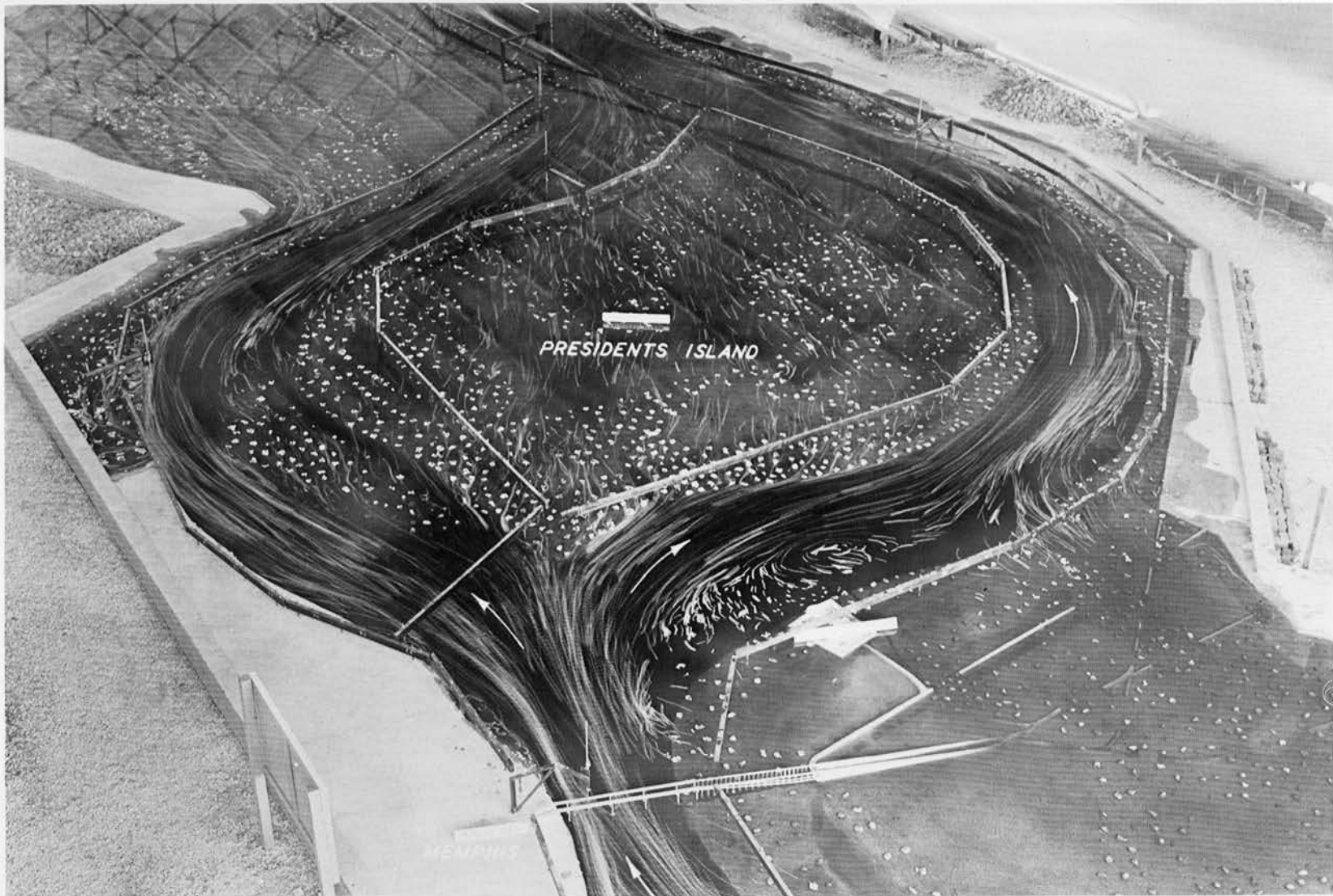
Photograph 5. Base Test 2 (existing conditions) with fixed-bed showing current directions at crest of project flood.
