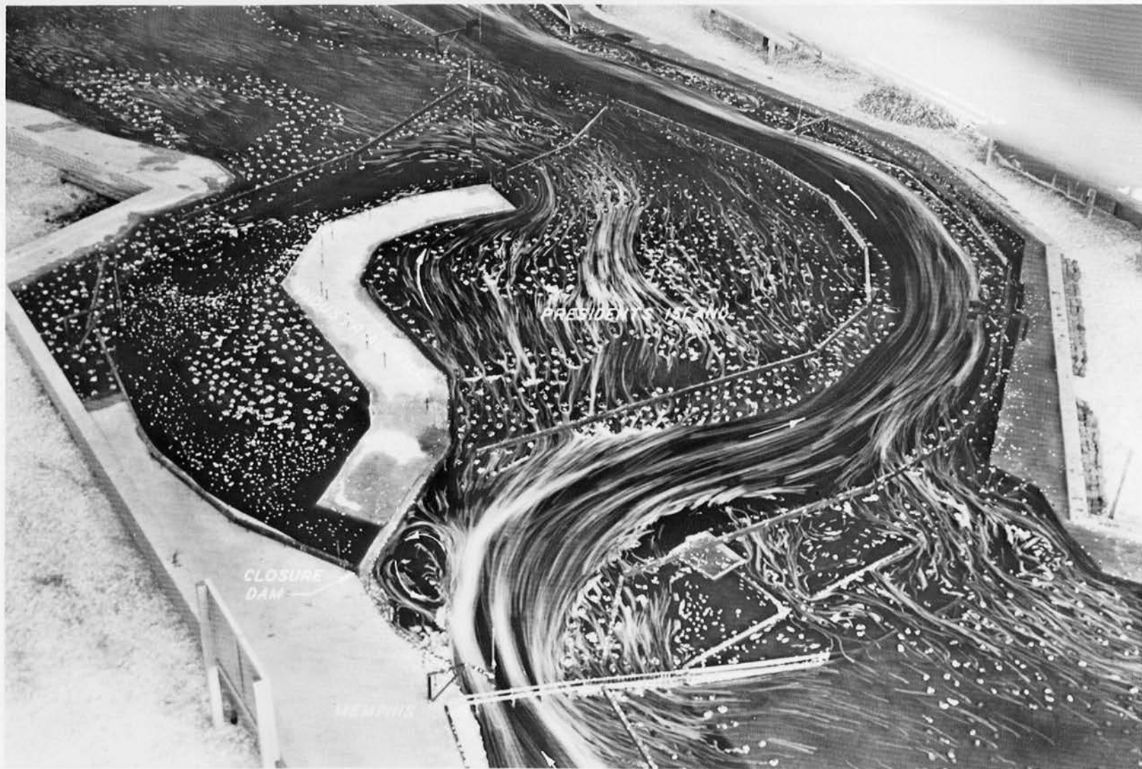
Photograph 4. Test 2 -- Plan 1 (left-bank chute levee removed) with fixed-bed showing current directions at crest of 1937 flood.
