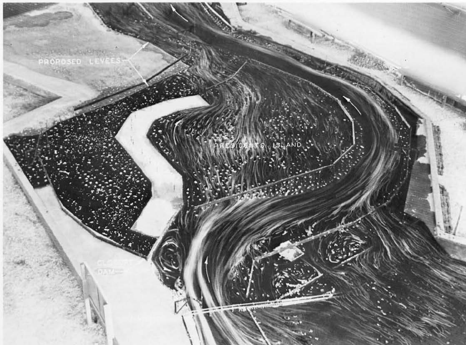
Photograph 6. Test 3 -- Plan 1 (entire improvement plan installed) with fixed-bed showing current directions at crest of project flood.
