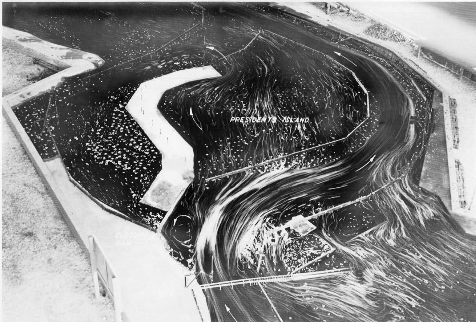
Photograph 7. Test 4 -- Plan 1 (left bank chute levee removed) with fixed-bed showing current directions at crest of project flood.
