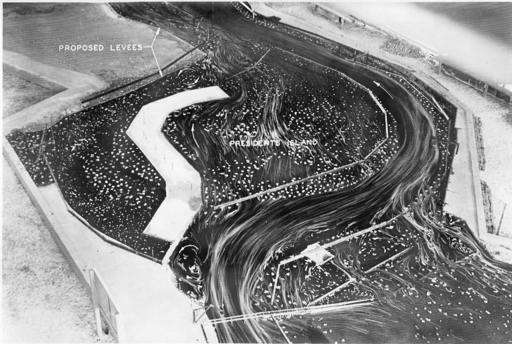
Photograph 3. Test 1 -- Plan 1 (entire improvement plan installed) with fixed-bed showing current directions at crest of 1937 flood.
