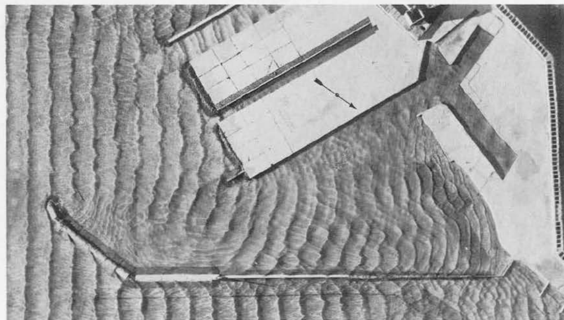
Figure 14. Plan U with 6.5-sec waves 15.5-ft high from south-southeast
