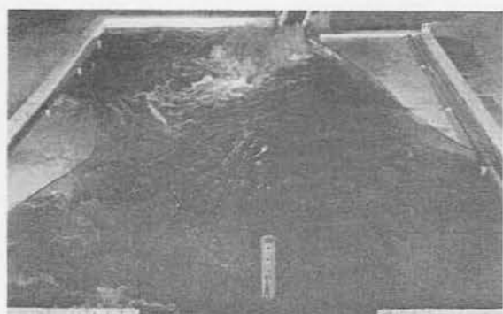
Fig. 10. Type E bucket; left wall elevation, 1570.0
