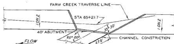
RIGHT BANK ABUTMENT PLAN 2
