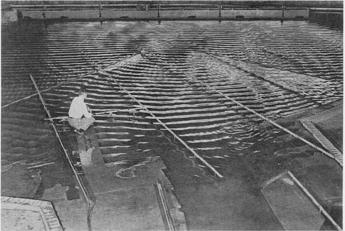
Fig. 1. General view of model; base-test conditions, 7-ft storm waves from north direction
