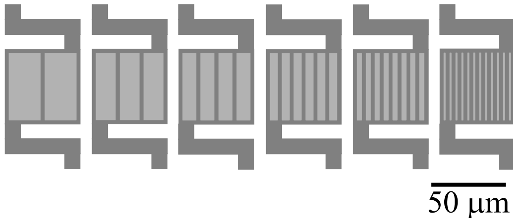
Figure 1. Different designs of regionally thinned microbolometers having 2, 3, 4, 6, 8 and 12 windows. The light gray regions are thinner than the dark gray regions.
