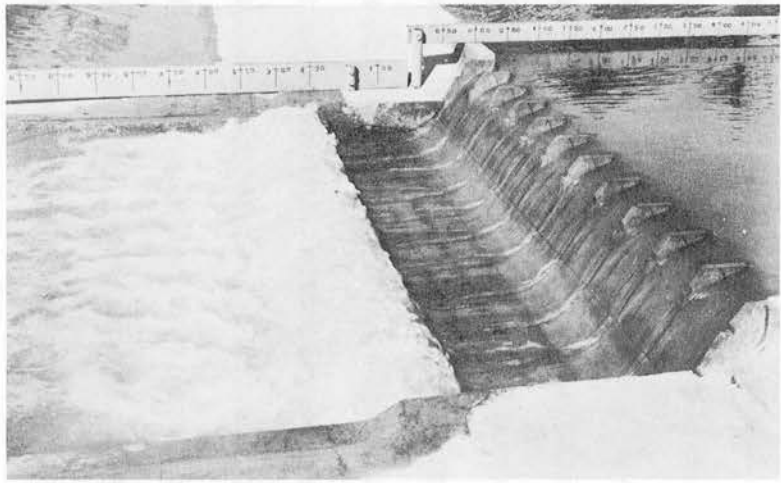
Discharge 462,000 cfs; tailwater elev 1899.5 Baffle piers removed from apron
