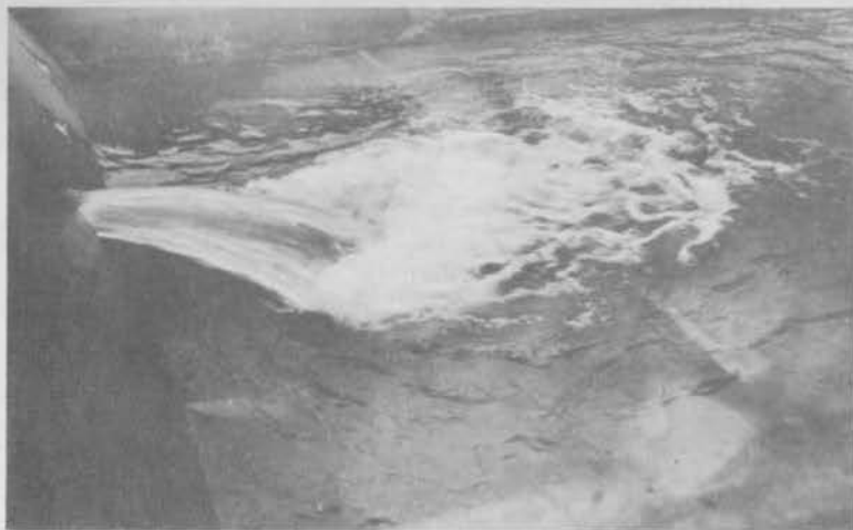
a. One sluice in operation Discharge 1,720 cfs Tailwater elev 491.3
