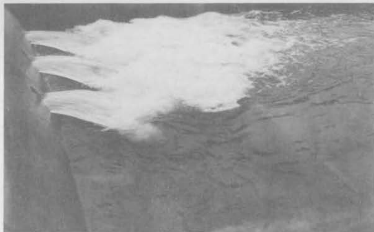
b. All sluices in operation Discharge 16,950 cfs Tailwater elev 496.7
