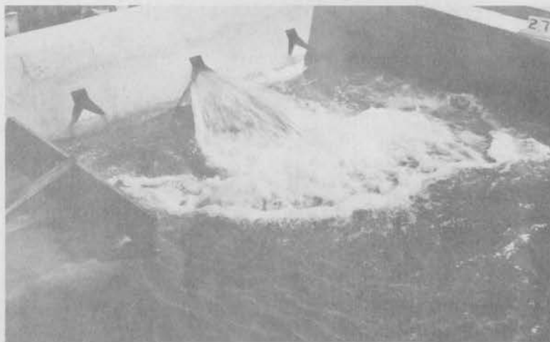
a. One sluice in operation Discharge 1,750 cfs Tailwater elev 491.3
