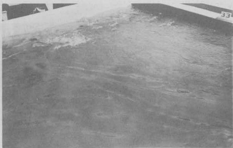
c. All sluices in operation Discharge 15,400 cfs Tailwater elev 511.5
