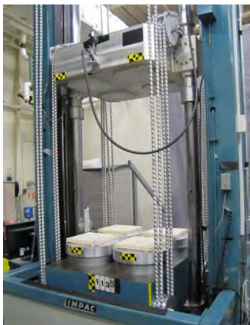
Figure 10. VID Facility with Installation of AFD and Felt Programmers
