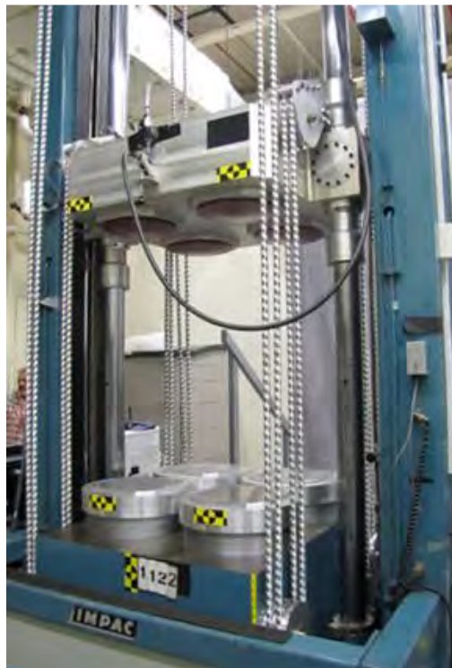
Figure 9. VID Facility with Installation of AFD and Red VID Programmers
