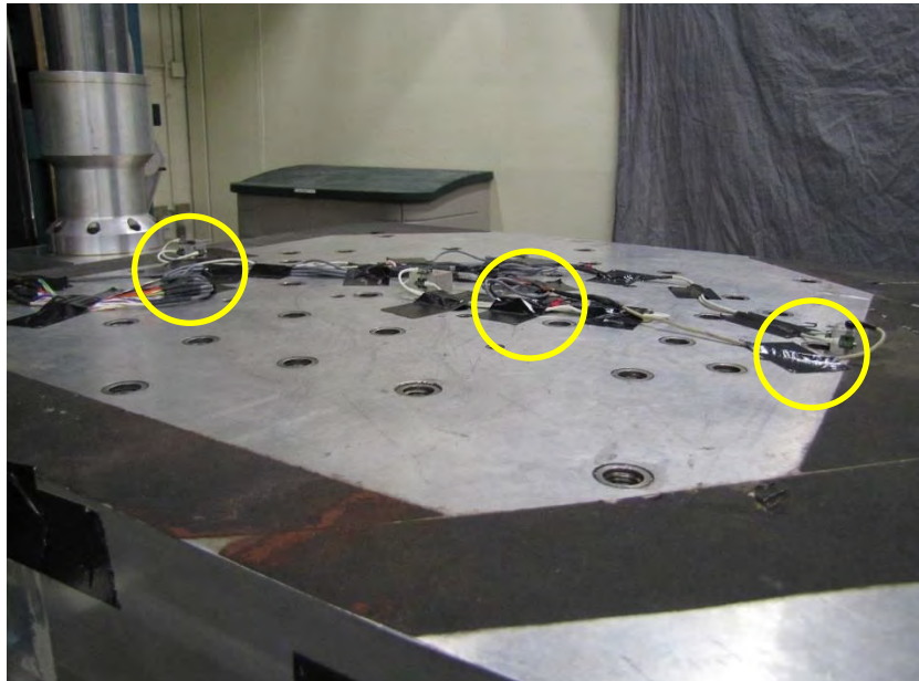
Figure 7. Location of Three Tri-axial Accelerometer Arrays on Top of VID Table
