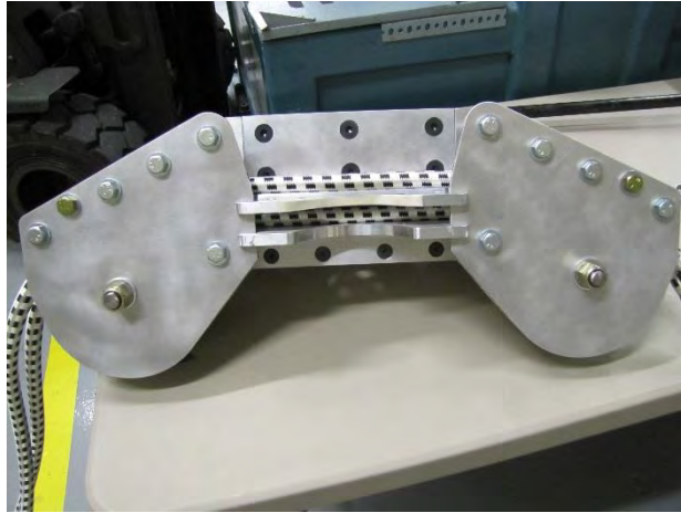
Figure 4. Side View of AFD Bungee Cord Guide Track
