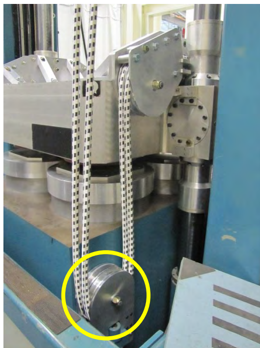
Figure 6. Installation of AFD Pulley Guide on VID Reaction Mass
