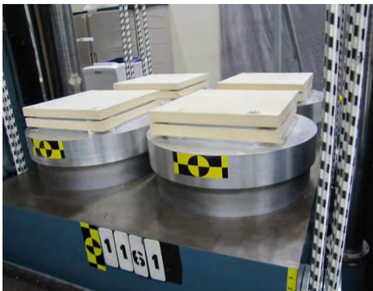
Figure 11. VID Facility with Installation of AFD and Felt/Plate/Felt Configuration
