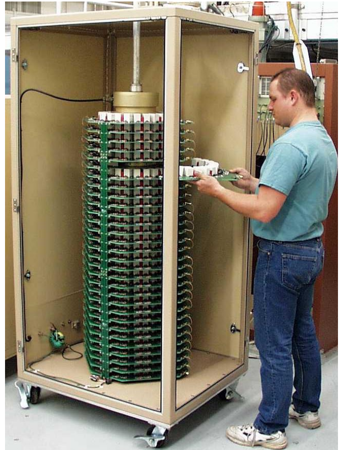
Figure 5. Kicker Pulser Assembly with MOSFET Carrier Boards Installed
