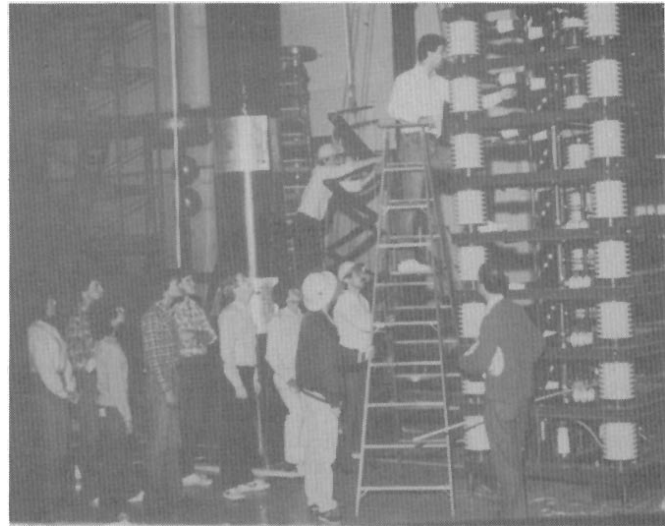
Figure 2 Graduate class preparing the 56 kJ, 3 MV Marx generator for laboratory experiments.
