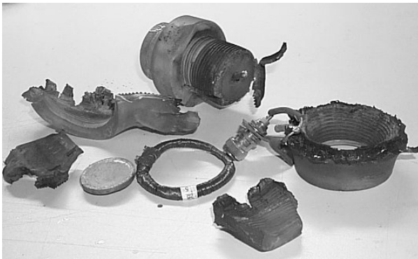
Figure 6. Explosive driven ferroelectric generator after the test.
