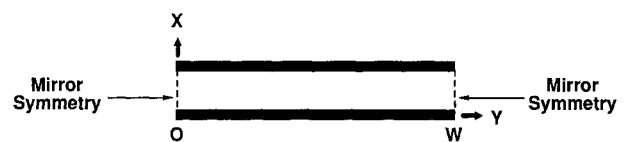
Figure 7. (a) The geometry a parallel-plate line.
