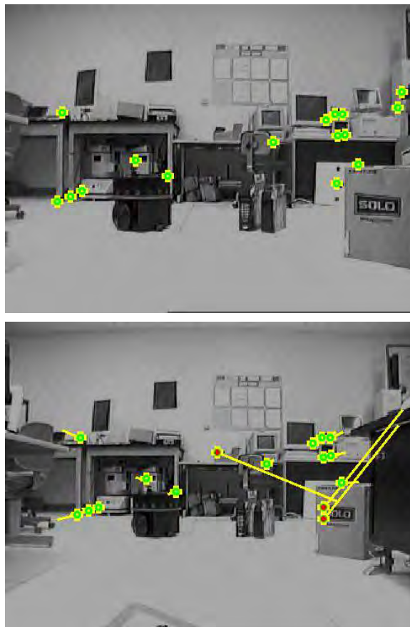
Figure 3: Two images in the linear sequence: Landmarks were selected in the upper image and recognized in the lower image. The lines denote correspondences. Note that in this pair, three mismatches occurred.
