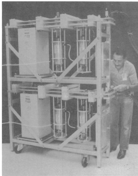
Fig. 1. Photograph of two 25-kJ modules.
