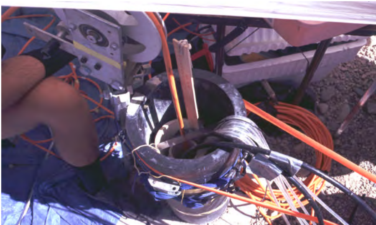
Figure 22. Photograph of geophysical logging (i.e., radar tomography) inside custom log-through packer and port system in well B4 during tracer/time-lapse imaging experiment at the BHRS in 2001. Note two lines for sampling head change with fiber-optic transducers, six lines for water sampling through a peristaltic pump, and one line for packer inflation – all coming from outside the riser but within the well.
