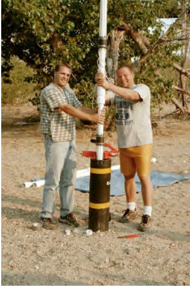
Figure 21. Photograph of custom log-through packer and port system with 1-m separations being assembled and installed in a well at the BHRS in preparation for the tracer/time-lapse imaging experiment in 2001.
