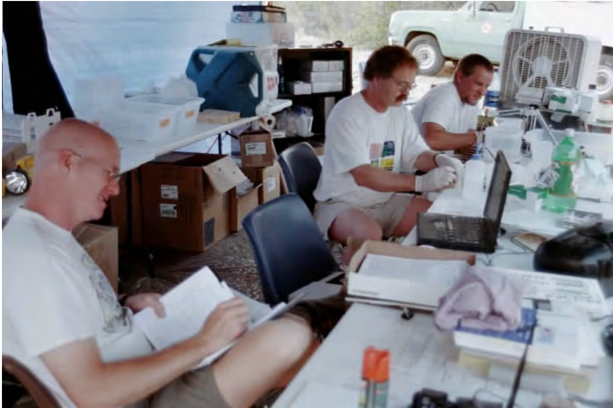
Figure 30. Photograph of the field chemistry laboratory at the BHRM which was used to generate near realtime results on uranine concentration from fluorescence and conductivity as analogue for bromide concentration from samples from 50 locations in six wells during the tracer/time-lapse imaging experiment.
