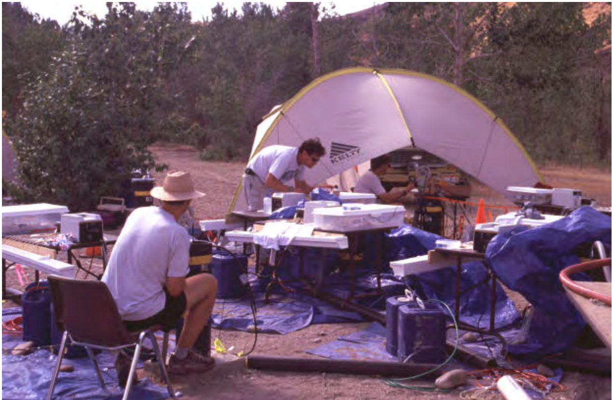
Figure 23. Photograph of sampling for water chemistry at well A1 in the middle of the radar imaging plane while radar tomography data are being collected through log-through packer and port systems in well B1 (near) and well B4 (far, under shade tent).
