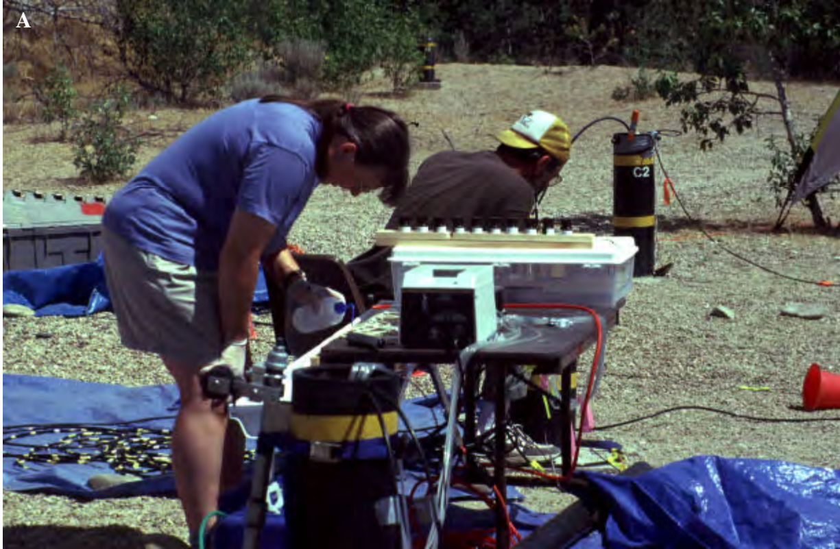
Figure 28. Photographs of sampling from a peristaltic pump drawing from 10 isolated zones in wells B1, B5, and B6.
