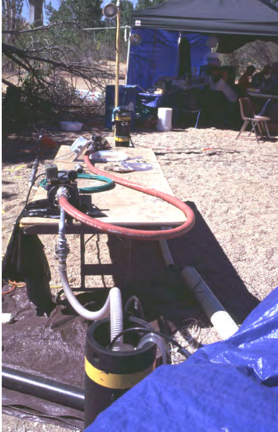
Figure 29. Photograph of discharge systems. Pumping from well B6 using log-through packer and port system with holes drilled into the center riser in zones of injection interval. Discharge was recorded with analogue and digital flow meters. Waste waters from continually-pumping peristaltic pumps and from the chemistry laboratory were collected in a drum (corner of field laboratory in background) and then pumped into the discharge line below flow meters.
