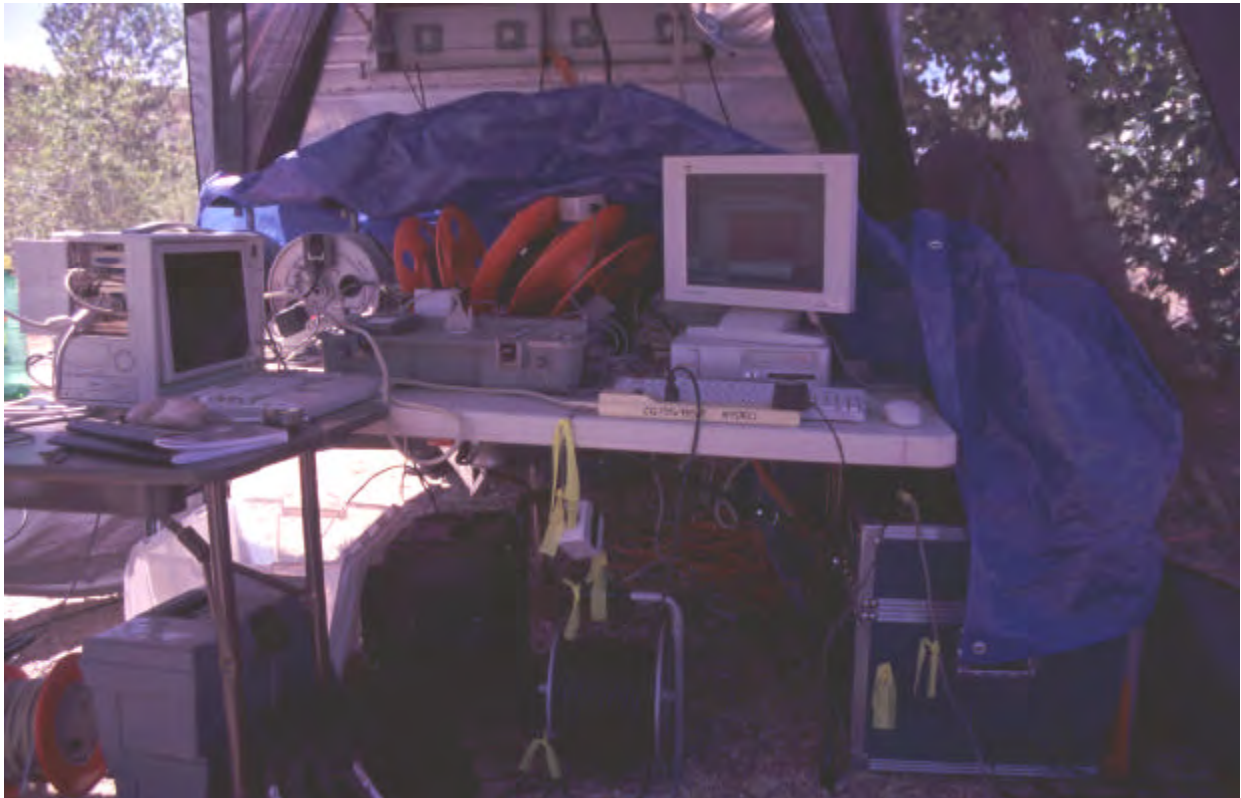
Figure 32. Photograph of station for logging head-change data from strain-gauge and fiber-optic transducers.
