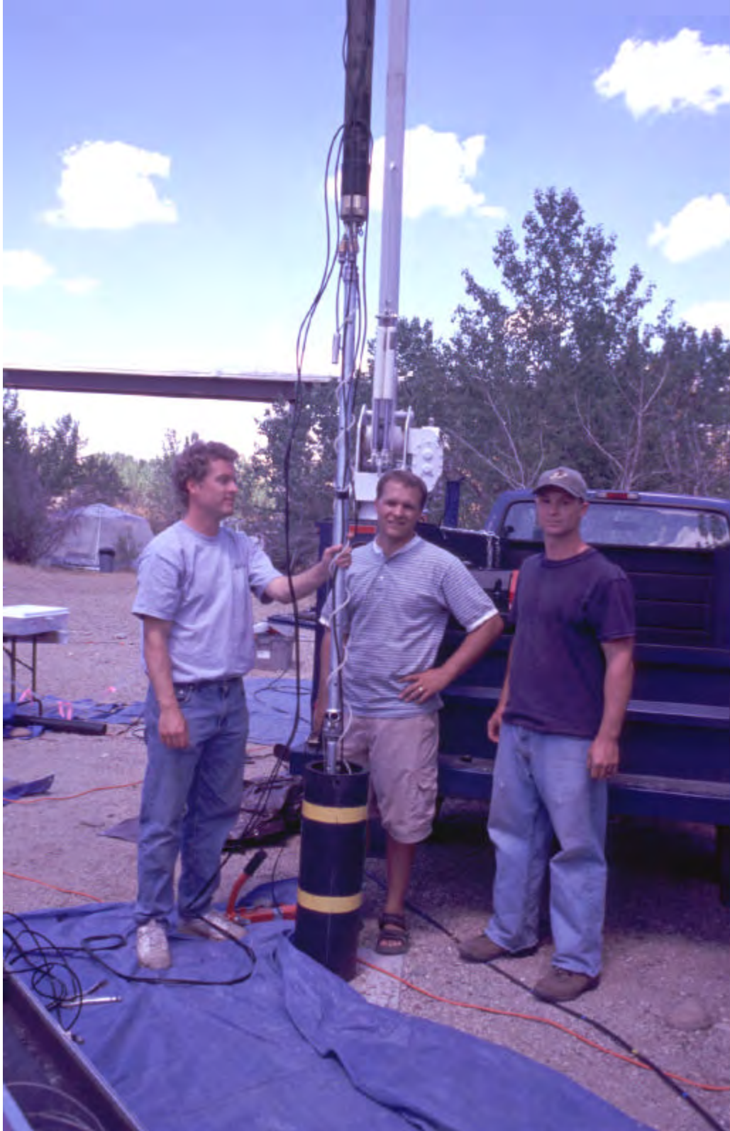
Figure 19. Photograph of straddle-packer being installed in well B3 showing upper portion of the injection zone and transducer for measuring head change within the injection zone.
