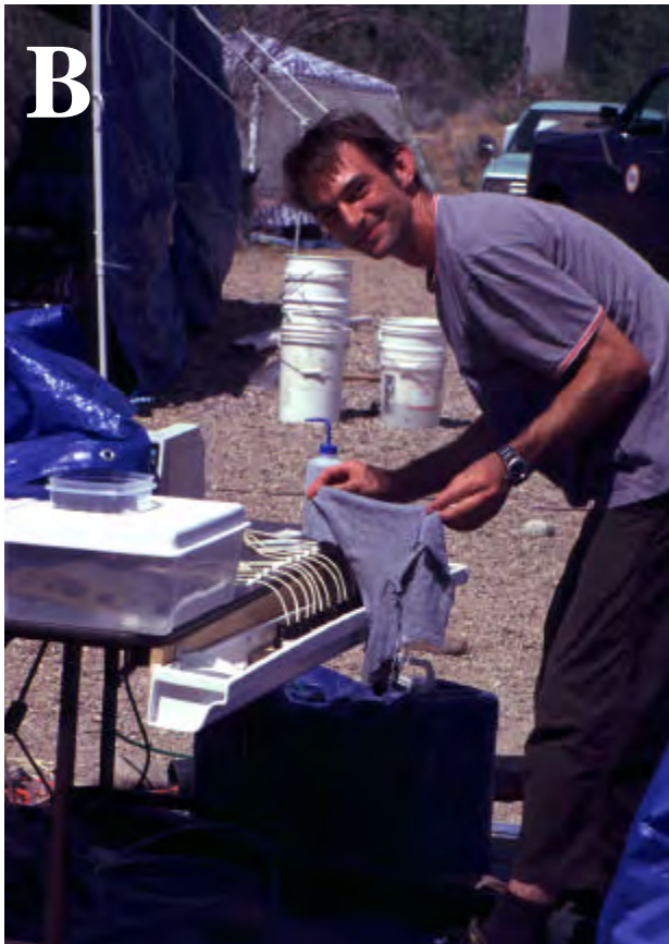
Figure 28. Photographs of sampling from a peristaltic pump drawing from 10 isolated zones in wells B1, B5, and B6.
