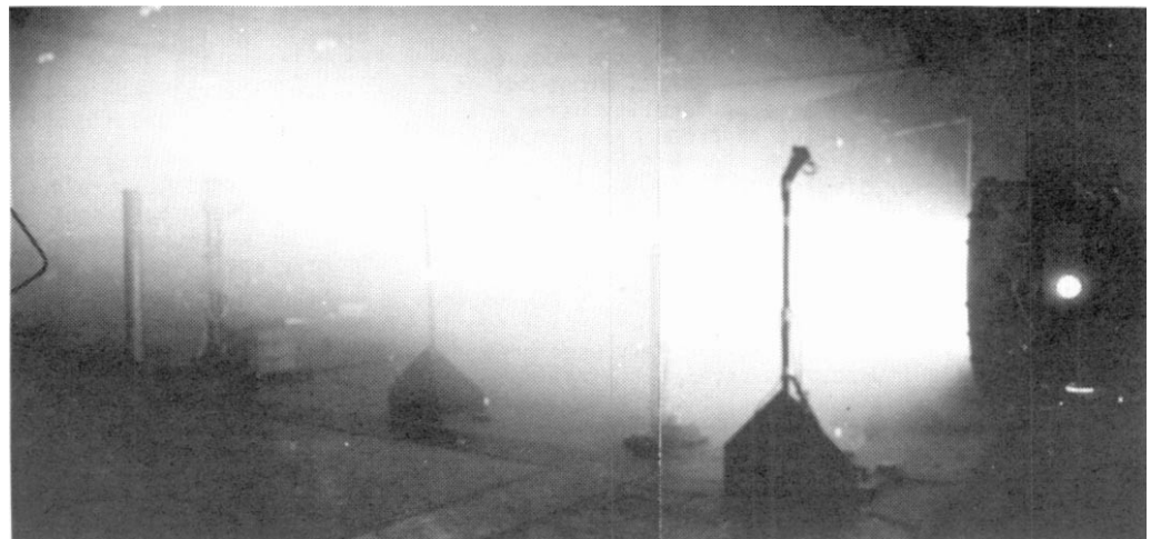
Figure 2. Electron Beam Traversing AURORA Test Cell.
