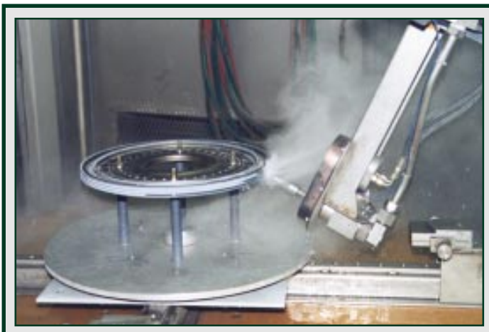
Removal of Flame Spray Coating Using UHPWJ
