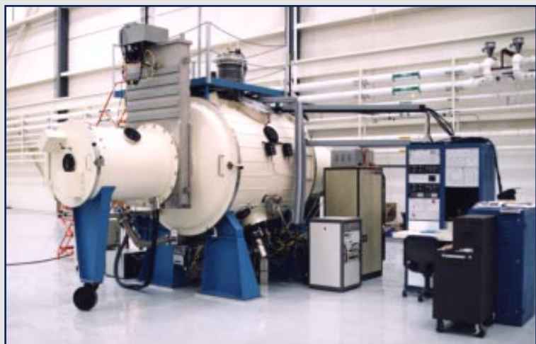
Ion Beam Assisted Deposition Chamber
