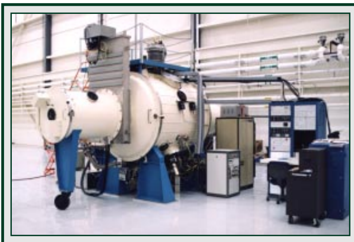
Located in the NDCEE Demonstration Facility, this technology has both ion implantation and ion beam assisted deposition capabilities.
