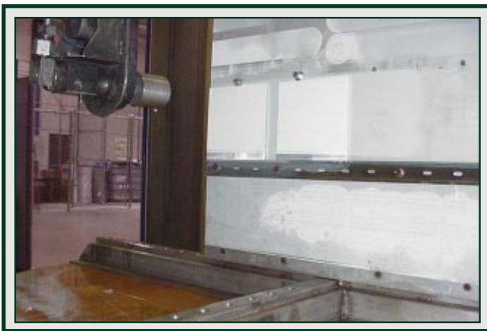
UHPWJ used for surface activation of aluminum adherends.
