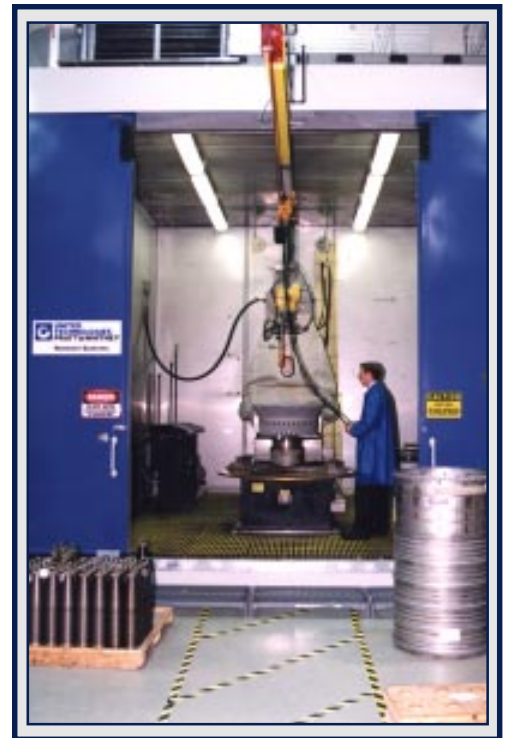
UHPWJ with robotic arm and turntable
