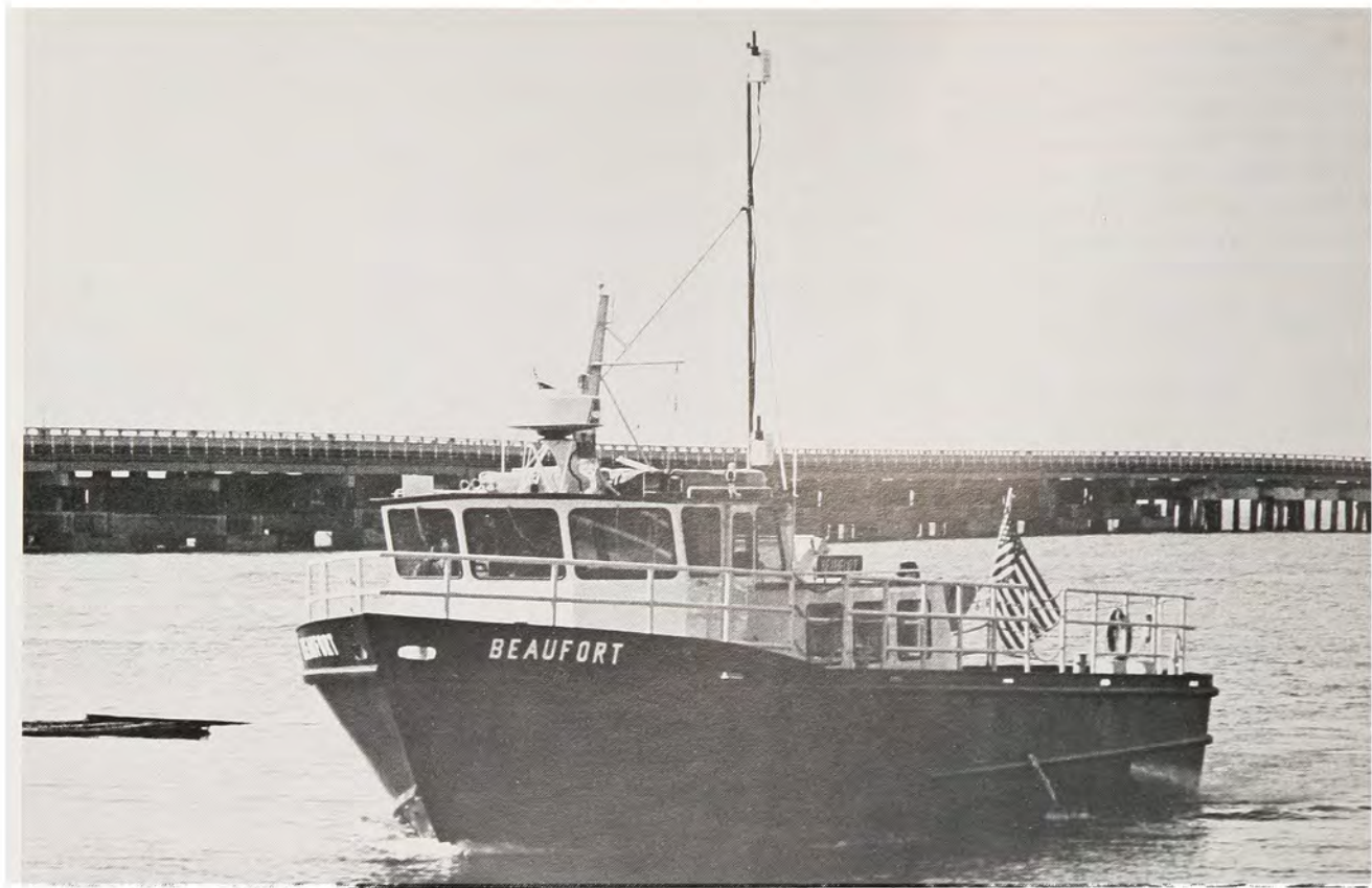
The Beaufort, a high-speed, 47-foot survey boat
