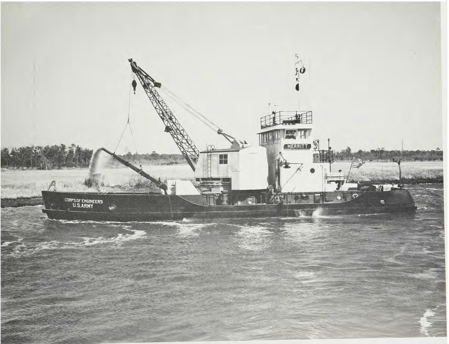
The Merritt after conversion to a sidescaster dredge, 1964
