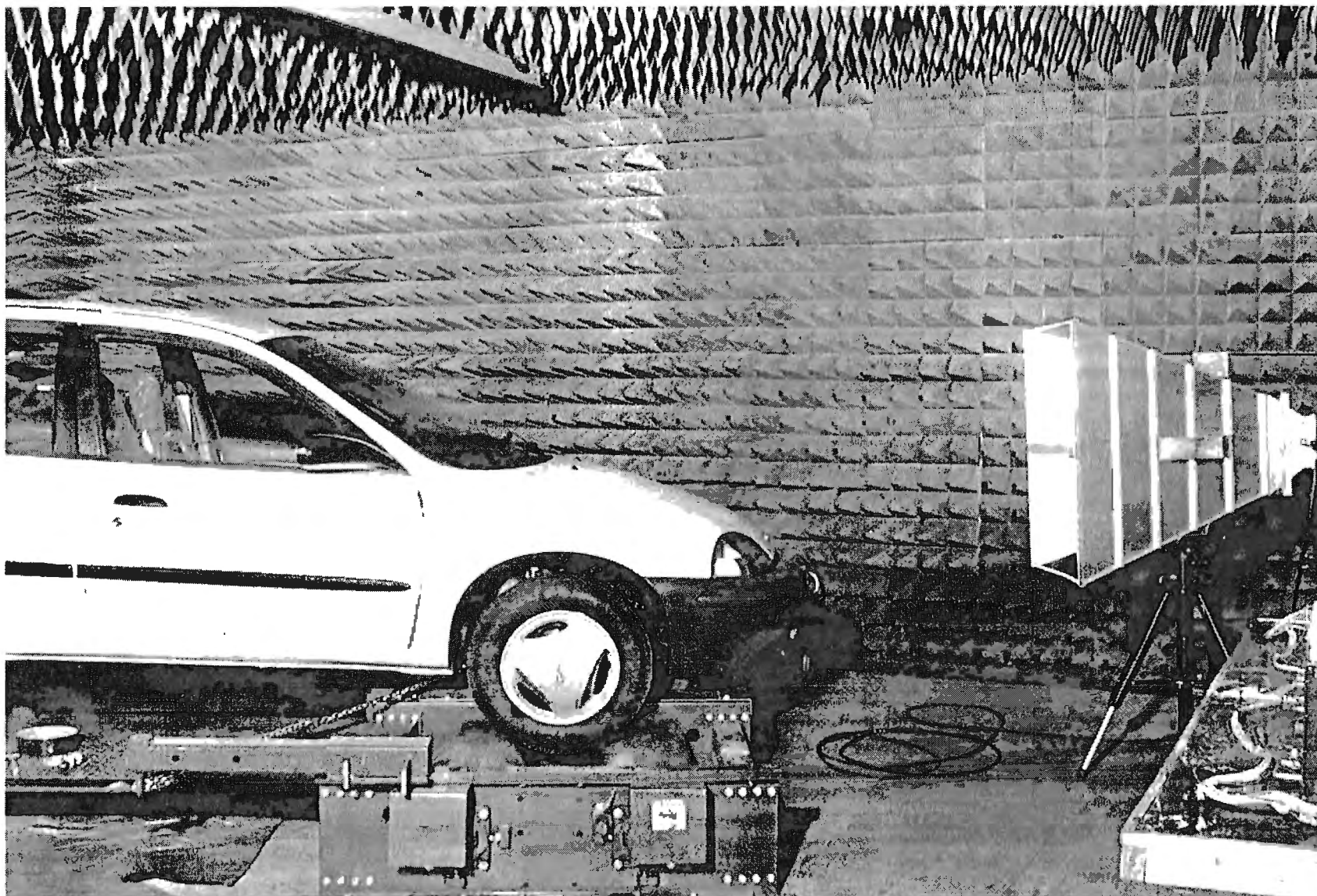
Figure 30. Solectria ICE Car in Anechoic Chamber Test
