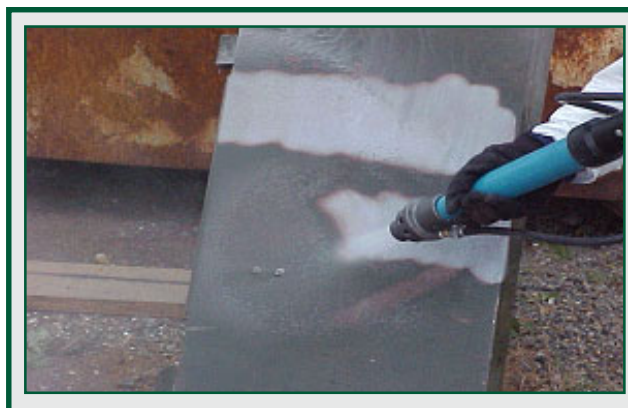
At NAB Little Creek, the NDCEE successfully field-demonstrated wet sodium bicarbonate blasting on an aluminum HMMWV component.
