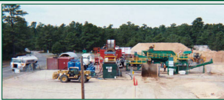
The NDCEE demonstration at Fort Dix showed that lead-contaminated range soils could be effectively treated in the field and the recovered metals could be recycled.
