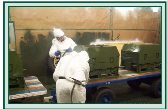
WD-CARC application at CEG-A Goose Creek
