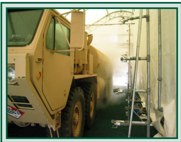
The portable Corrosion Prevention and Control System automatically cleans vehicles, such as this Heavy Expanded Mobility Tactical Truck, and then applies a corrosion inhibitor for metal protection.
