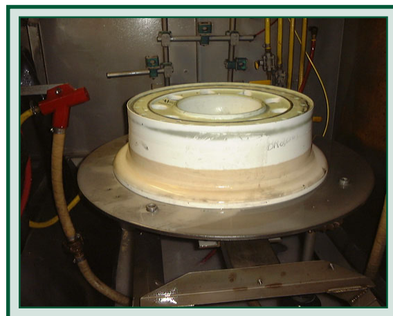
Aluminum oxide wet slurry blasting using 3/0 quartz
