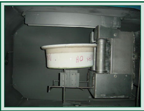
Landing gear wheel mounted in a motorized ZCW airless test machine
