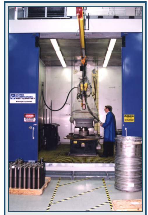
UHPWJ with robotic arm and turntable
