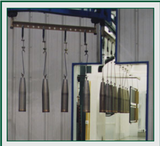
Automated powder application to 105-millimeter artillery projectiles
