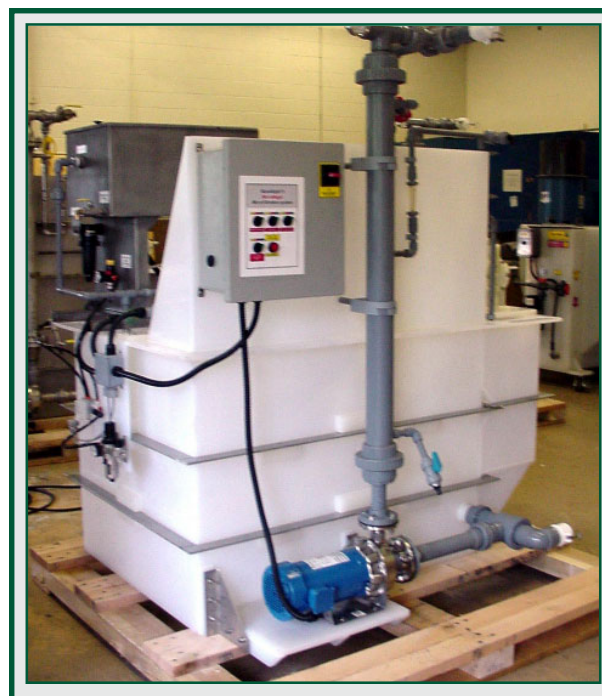
Microfiltration system housed at the NDCEE Demonstration Facility
