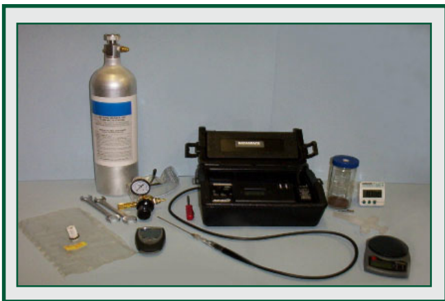
X-Wand portable test kit components for HVOC field screening
