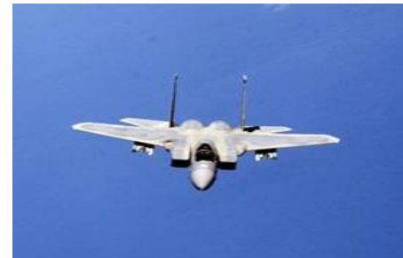
THE F-15 IS ARMED WITH THE AIM-7M SPARROW OR AIM-120 ADVANCED MEDIUM-RANGE AIR-TO-AIR MISSILES, THE AIM-9M SIDEWINDER, AND A 20-MILLIMETER CANNON.
