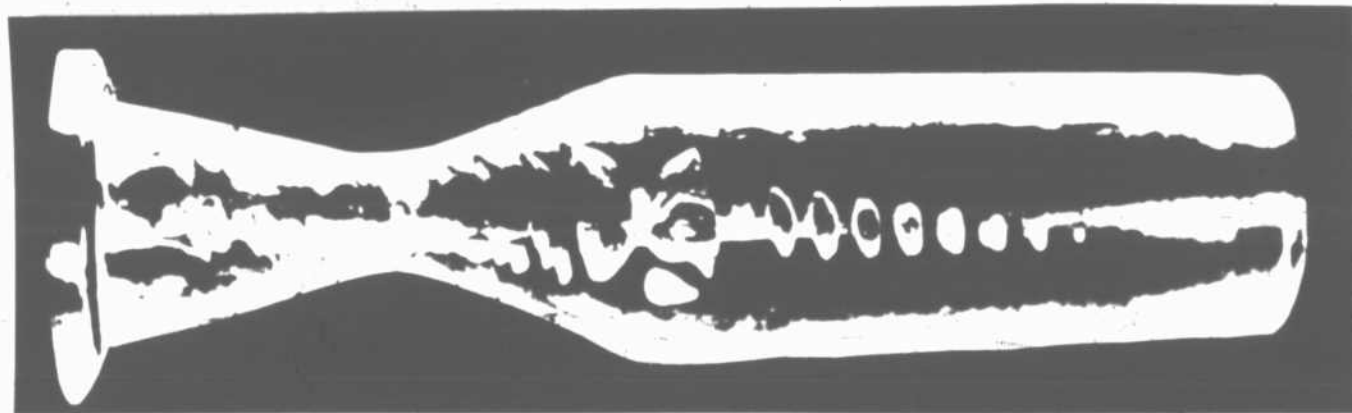
Fig. 12 - Formation of Dark Spots After Half-Hour Run With Injector Distribution No. 1
