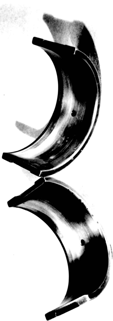
FRONT INTERMEDIATE MAIN BEARING AFTER 150 HOURS ENDURANCE PRATT & WHITNEY XR-4360-4 ENGINE
