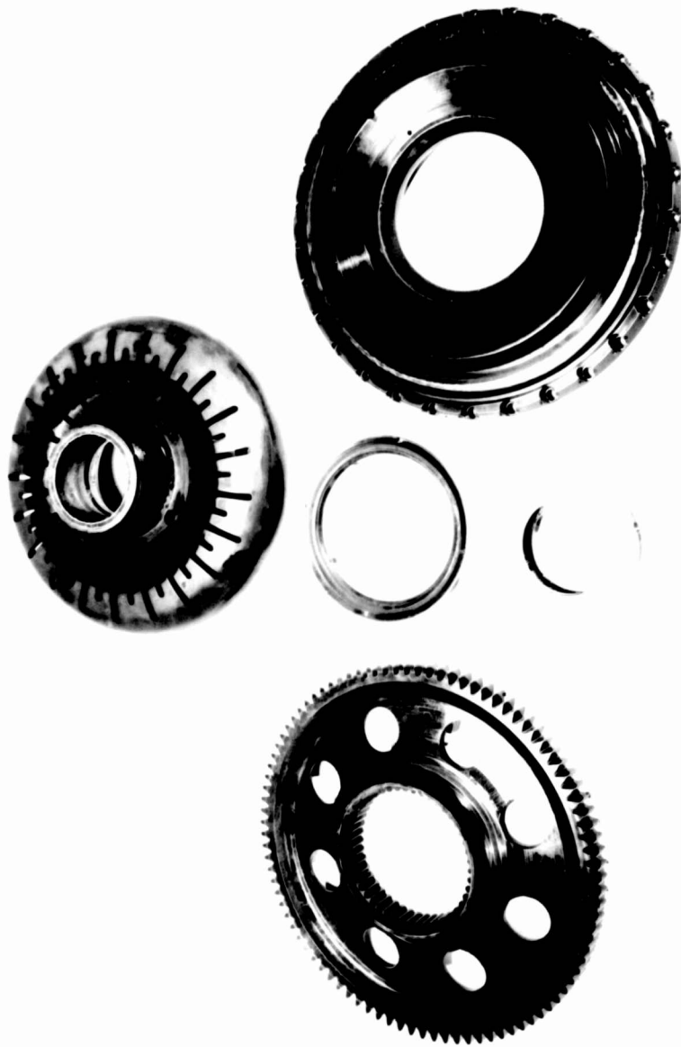
LEFT COUPLING - VARIABLE SPEED DRIVE AFTER 77 HOURS ENDURANCE PRATT & WHITNEY XR-4360-4 ENGINE
