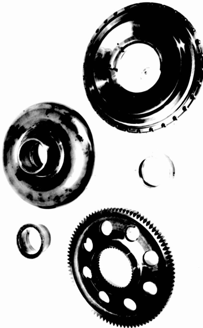
RIGHT COUPLING - VARIABLE SPEED DRIVE AFTER 77 HOURS ENDURANCE PRATT & WHITNEY XR-4360-4 ENGINE
