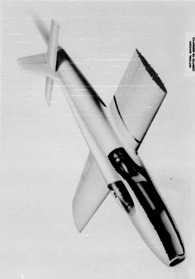
Figure 1.- High-speed subsonic jet-propelled airplane with a proposed duct for the air-induction system.
