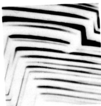
FIG.7. SILVER HEATED IN AIR 11 HRS. 920° C (X 2,000)
