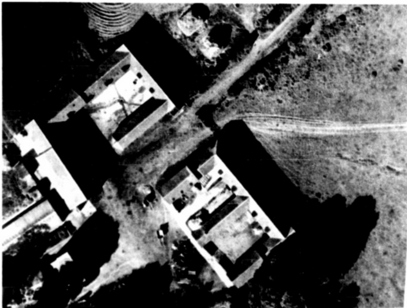
B. EXPERIMENTAL FINE GRAIN FILM: f/11: 1/70 SEC: MINUS BLUE FILTER: MOVING FILM MAGAZINE: GYMBAL MOUNTING.
